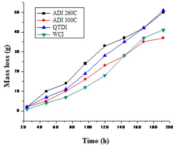
Figure 5 – Accumulated mass loss of the samples.
