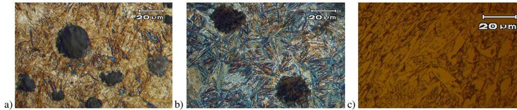
Figure 4 - Metallographic representation of the samples: a) QTDI, b) ADI 300<sup>o</sup>C and c) WCI.
