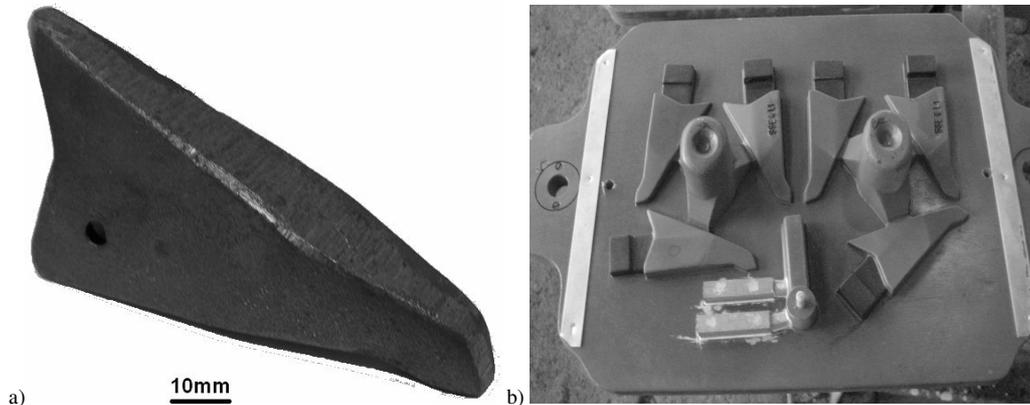
Figure 1 - Aspects of the wear test: a) format of the wear specimen and b) plate model for molding.
