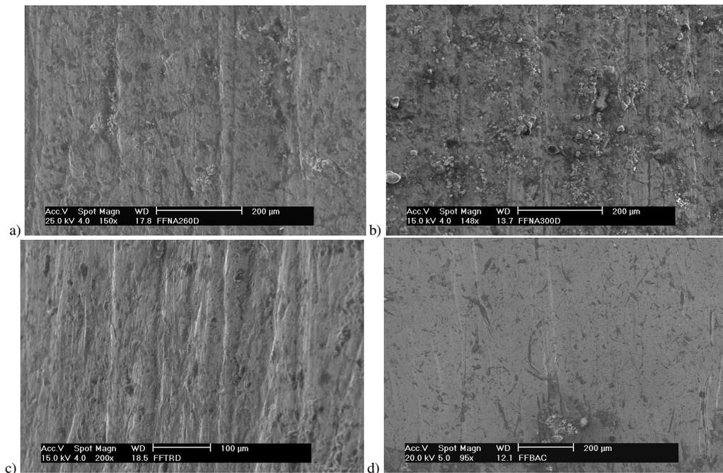
Figure 7 - Appearance of surface samples: a) ADI 260<sup>0</sup>C, b) ADI 300<sup>0</sup>C, c) QTDI and d) WCI.
