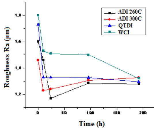
Figure 6 - Comparison of the roughness Ra of the samples tested.
