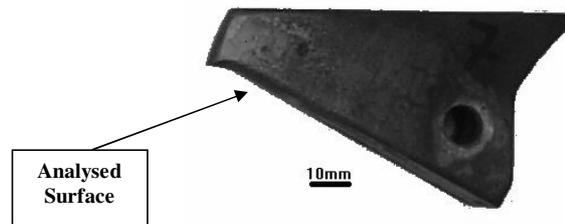
Figure 3 - Position of the assessment of surface roughness.
