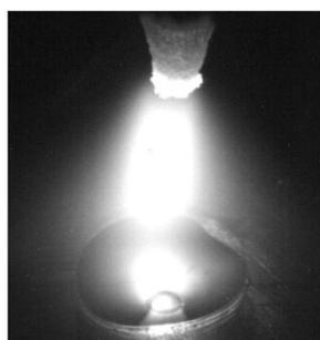
Figure 2. GTAW in carbon steel, Argon, 100 A, with a optic long pass filter in 850 nm (VILARINHO, 2009).
