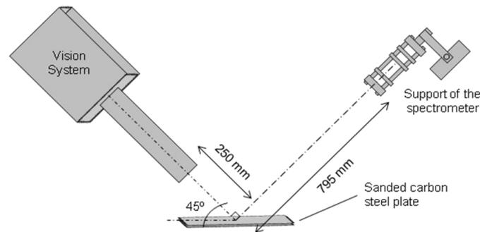
Figure 8. Experimental setup to study the emission NIR of the vision system with laser diodes.
