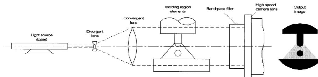
Figure 1. View of metal transfer by back-lighting technique (BÁLSAMO *et al.*, 2000)
