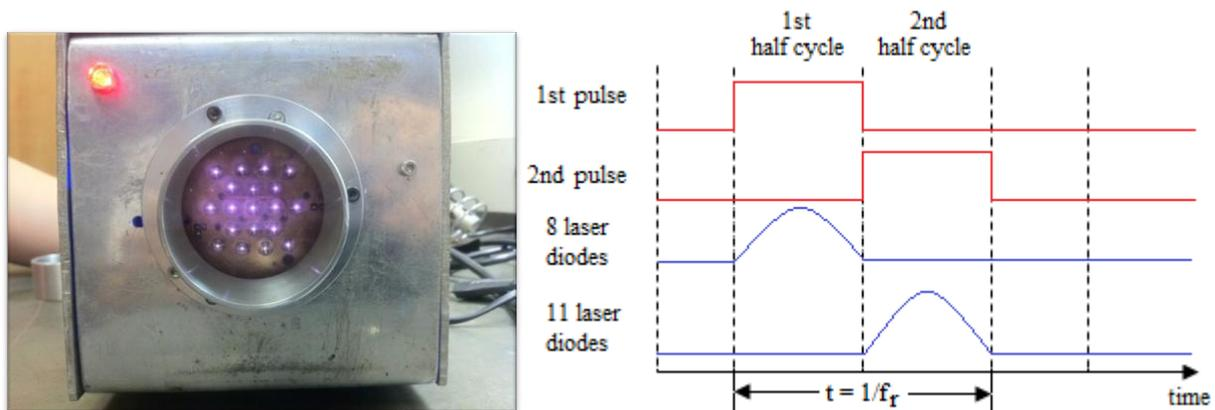
Figure 5. Vision system: set of 19 driven laser diodes (left) and schematic functioning of the circuits (right).
