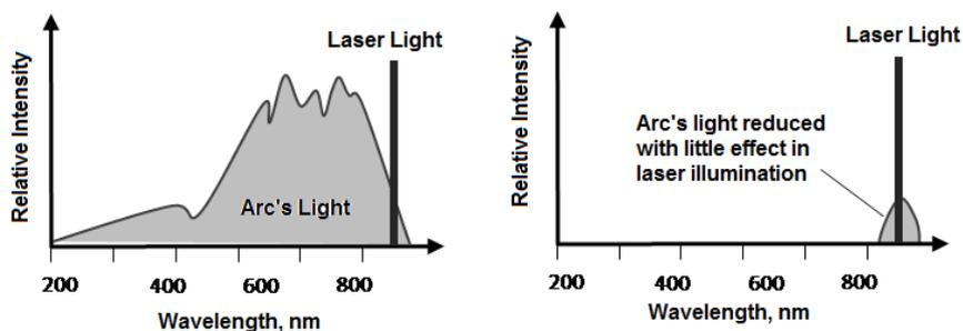
Figure 3. Principle of Spectrum Filtering (HOUGHTON *et al.*, 2007).
