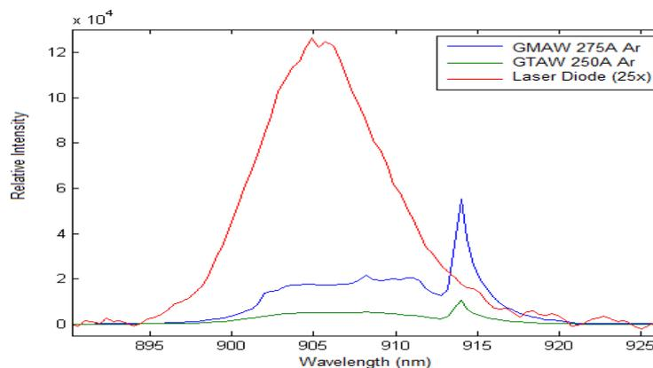
Figure 11. Comparison of the spectra of welding processes and the vision system.
