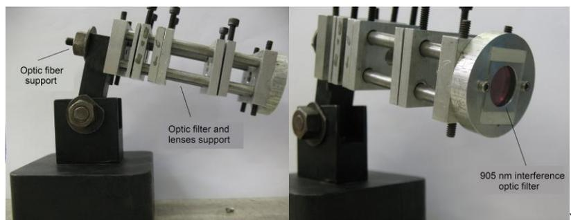
Figure 6. Support to optic fiber and lenses (left) and detail to the band pass filter (right).
