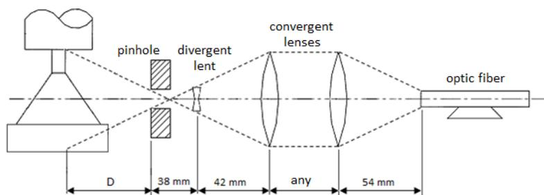
Figure 7. System of lenses used to focusing the arc in the optic fiber.
