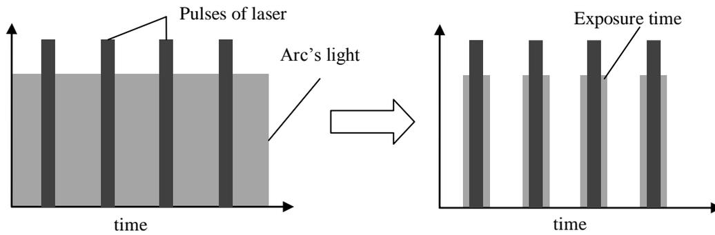
Figure 4. Exposure time adjusting to minimize the power applied to the laser.
