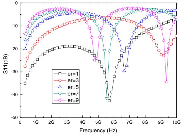
Figure 2. Magnitude S11 as a function of frequency.
