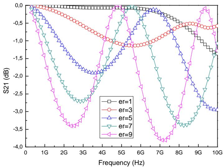
Figure 3. Magnitude S21 as a function of frequency.
