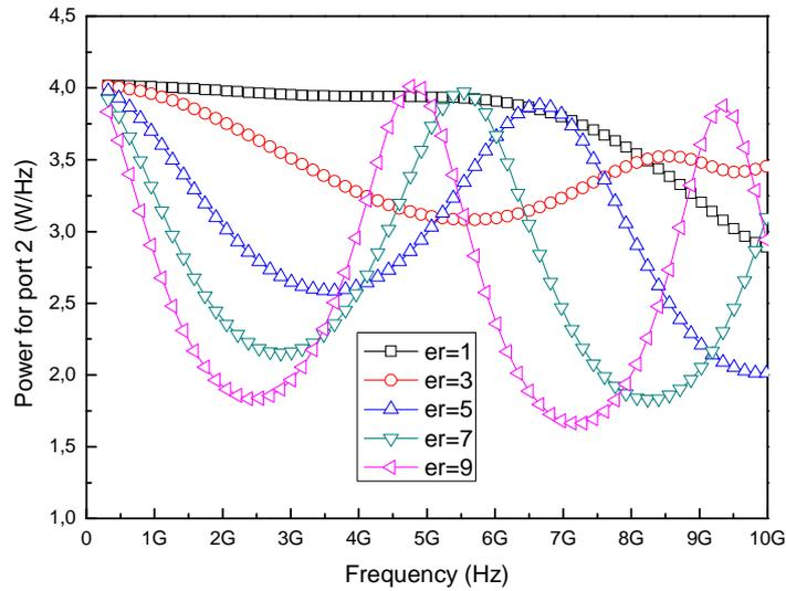
Figure 7. Power for port 2 in function of the frequency.
