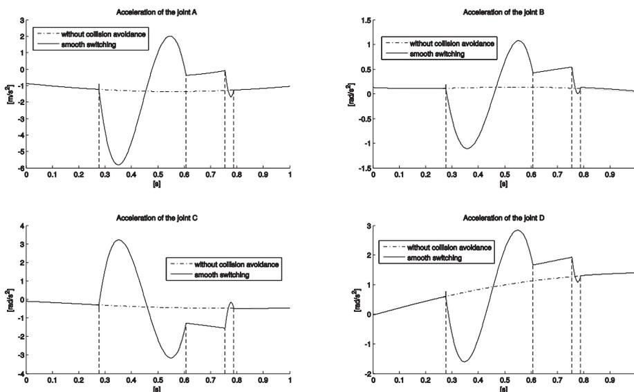
Figure 5. Accelerations of the joints *A*, *B*, *C* and *D*
