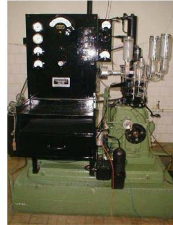
Figure 1 – CFR engine
