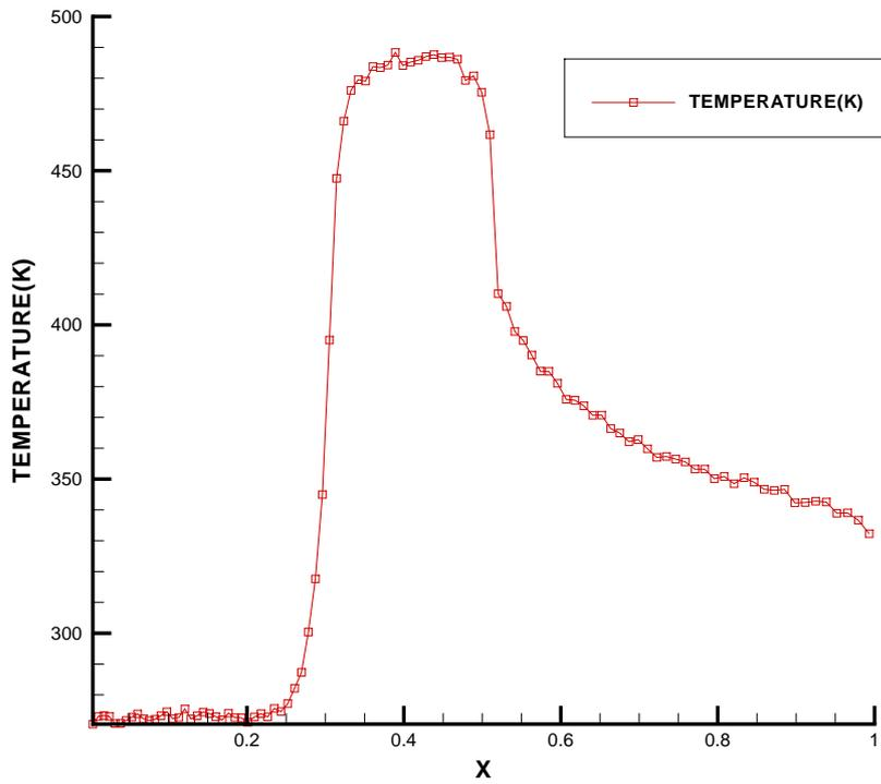
Figure 11. Temperature distribution profile throughout the flat plate configuration for free stream Mach number 2.4.
