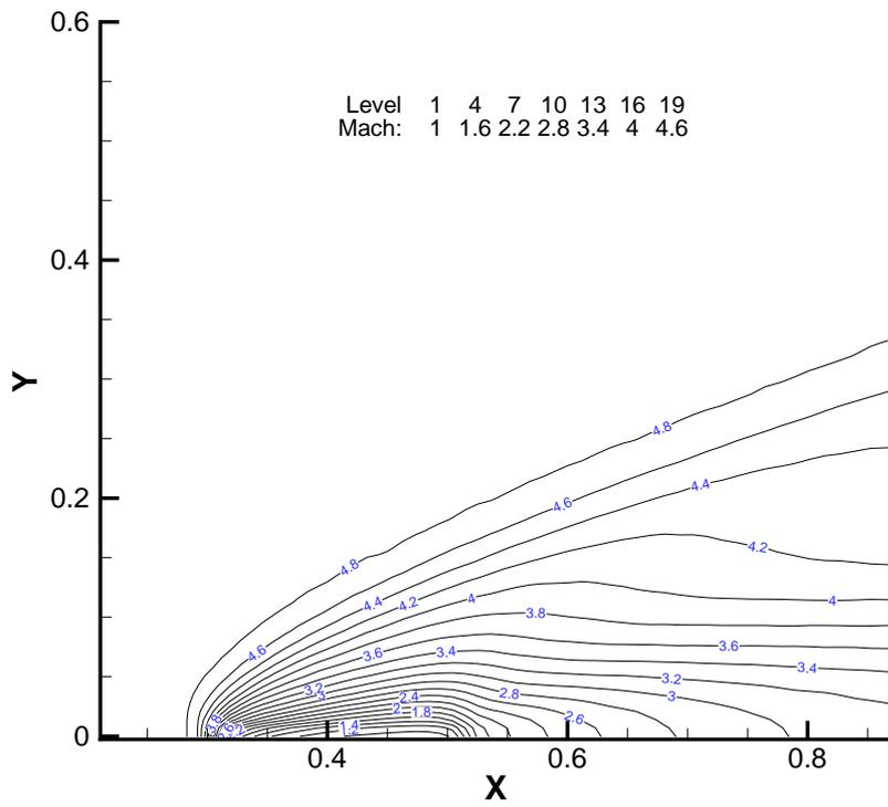
Figure 6. Mach number contours in the flat plate configuration for free stream Mach number 4.8.
