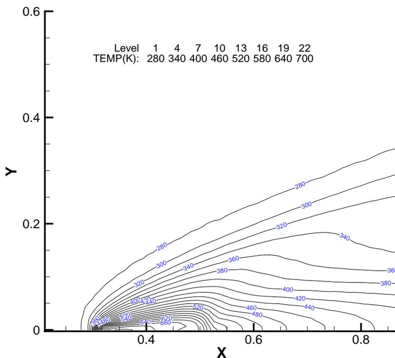
Figure 5. Temperature contours in the flat plate configuration for free stream Mach number 4.8.
