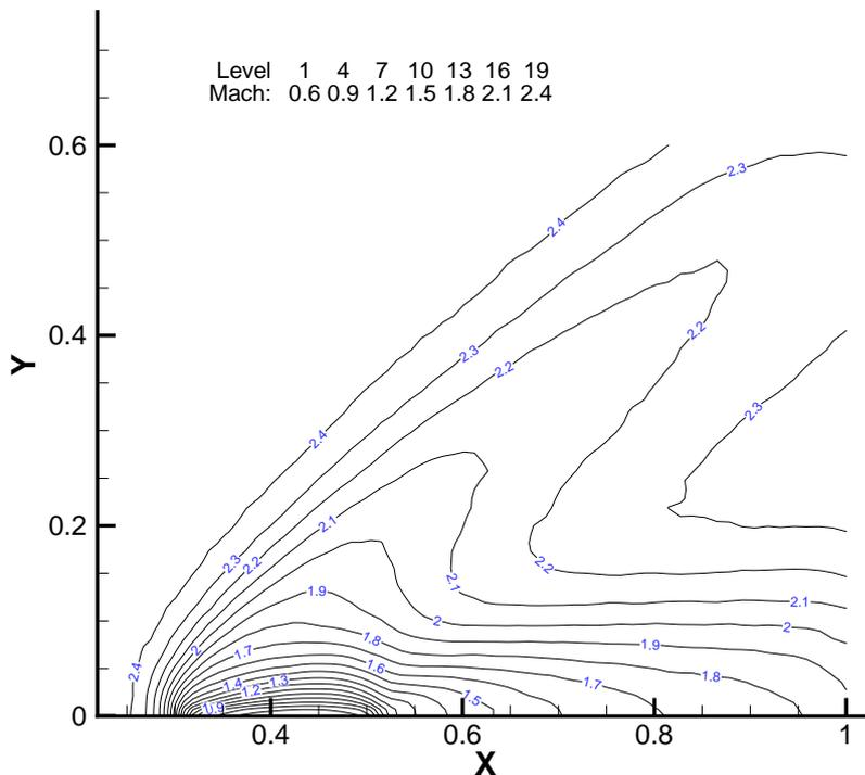
Figure 10. Mach number contours in the flat plate configuration for free stream Mach number 2.4.
