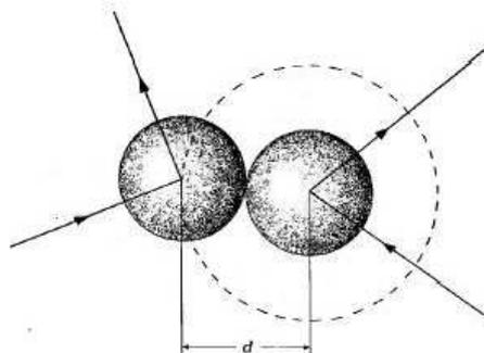
Figure 2. Collision cross section  $\sigma_T$  between two hard spheres of diameter  $d$ .
