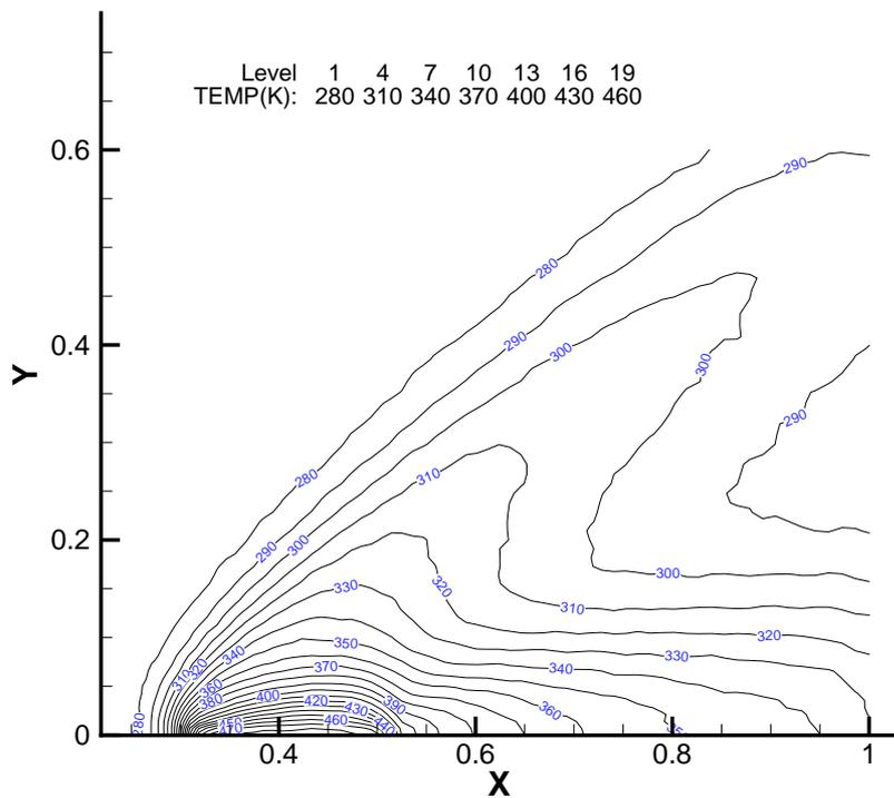
Figure 9. Temperature contours in the flat plate configuration for free stream Mach number 2.4.
