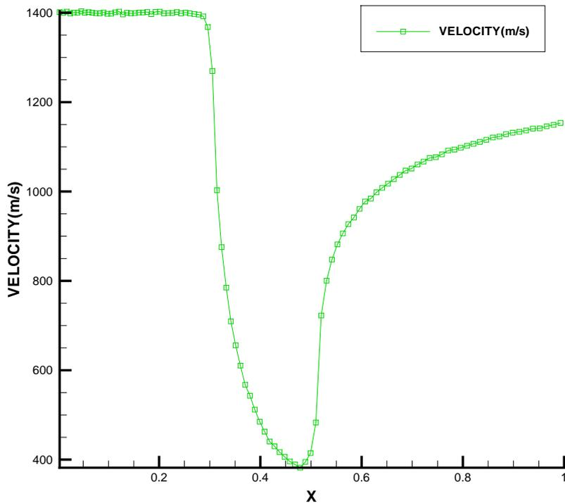
Figure 8. Velocity distribution profile throughout the flat plate configuration for free stream Mach number 4.8.
