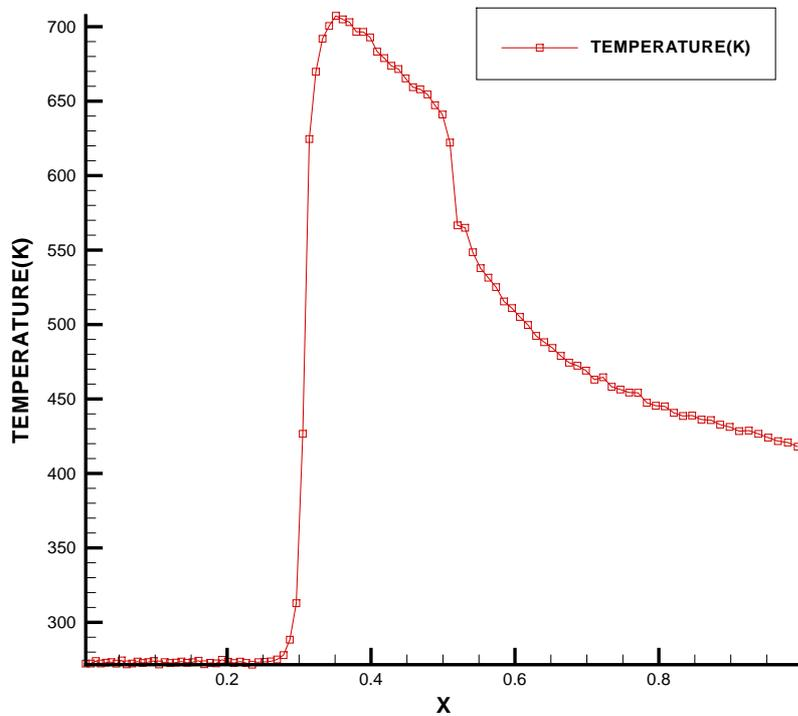
Figure 7. Temperature distribution profile throughout the flat plate configuration for free stream Mach number 4.8.
