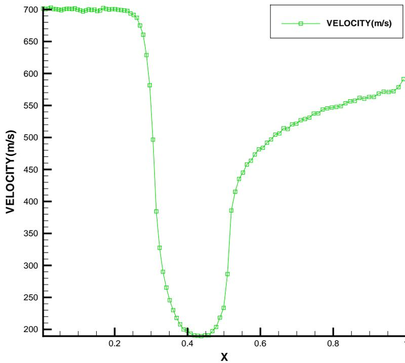
Figure 12. Velocity distribution profile throughout the flat plate configuration for free stream Mach number 2.4.
