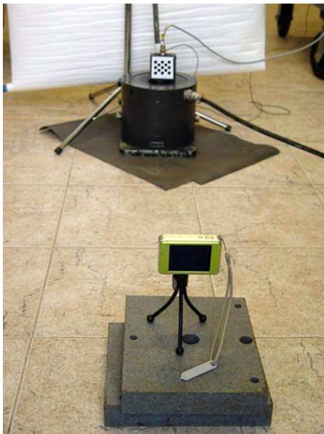
Figure 2. Set-up for testing one-dimensional vibration measurement (shaker movements).
