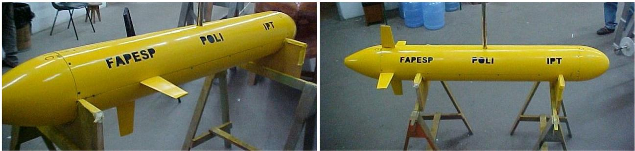
Figure 8. Captive model of Maya (left side) and Pirajuba (right side) wing-body combination.
