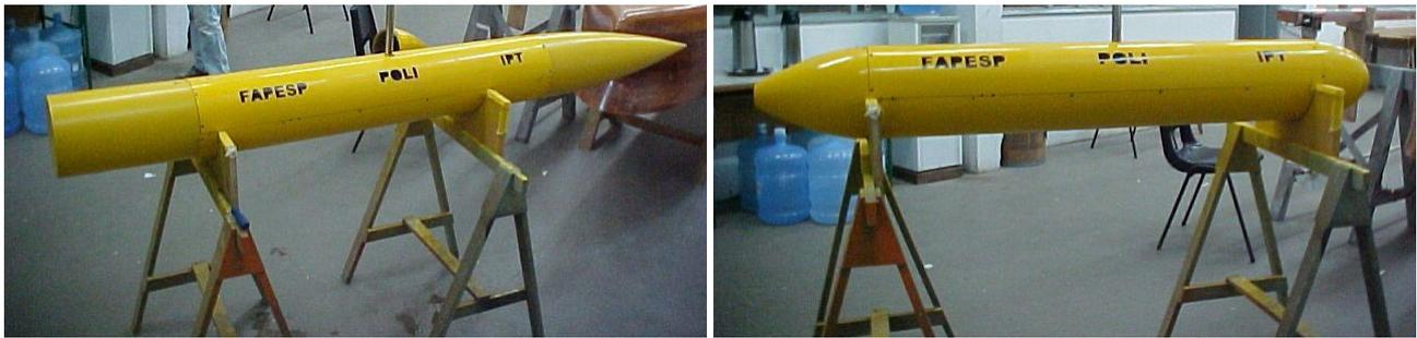
Figure 2. Models tested in IPT towing tank. NACA missile (Jorgensen, 1977) in the left side (a), and Maya/Pirajuba bare hull in the right side (b).
