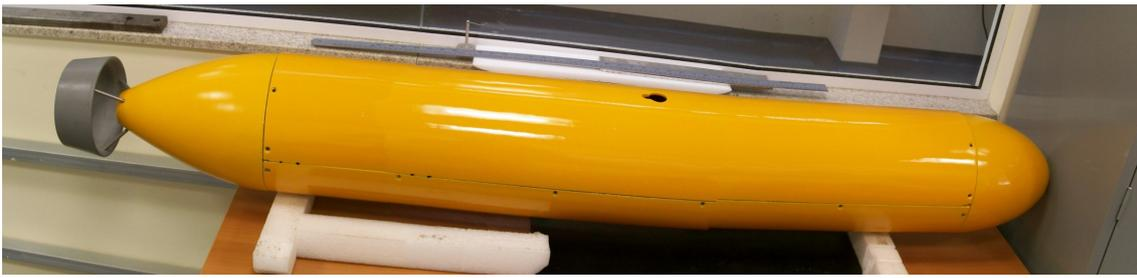
Figure 6. Captive model of AUV Pirajuba bare-hull with a propeller duct.
