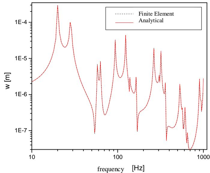
Figure 7 - Transversal displacement  $W$  on plate 2. Comparison between the analytical model and the Finite Element Model.
