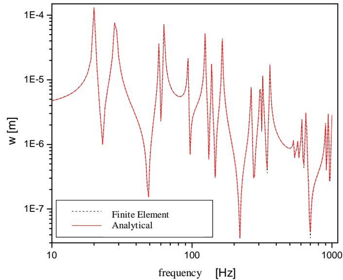
Figure 6 - Transversal displacement  $W$  on plate 1. Comparison between the analytical model and the Finite Element Model.
