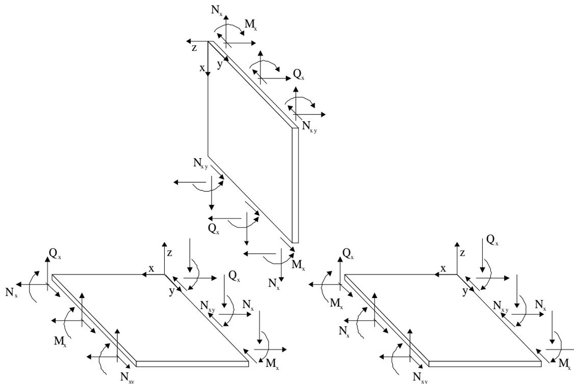
Figure 4 – Loads acting on plates 1, 2 and 3.
