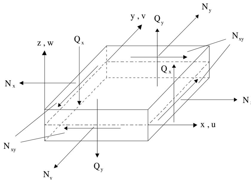
Figure 2. Thin plate submitted to in-plane loads.
