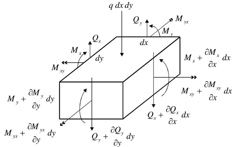
Figure 1. Thin plate element submitted to forces and moments.
