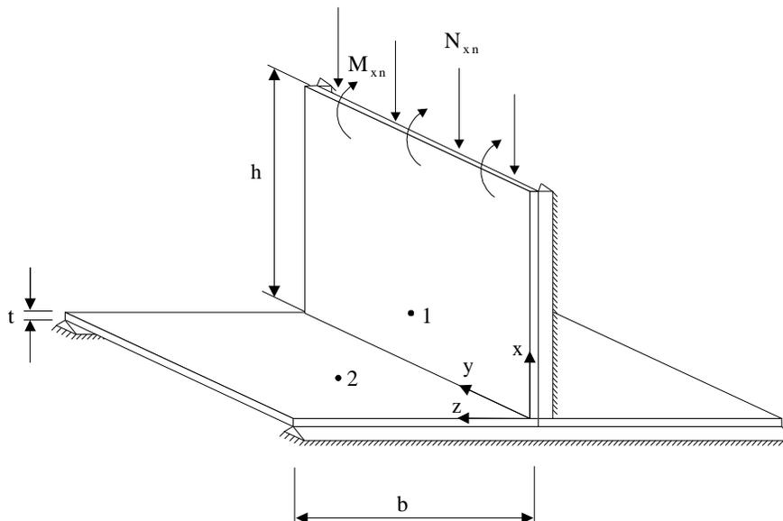
Figure 5 – Three coupled plates in a T configuration.
