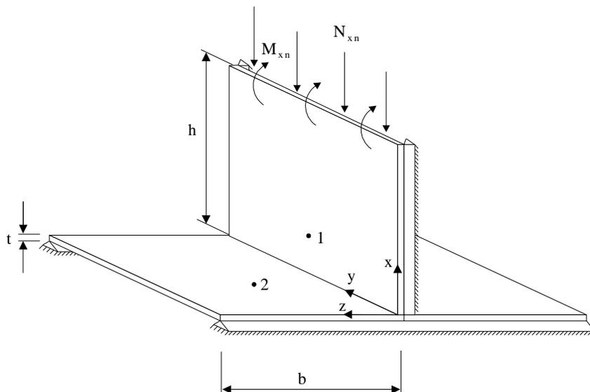
Figure 3 – Three coupled plates in a T configuration.
