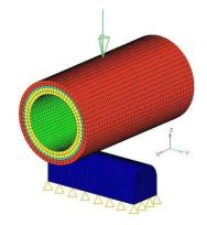
Figure 9. Model of the riser with internal pressure.
