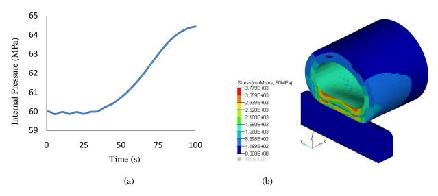
Figure 10. (a) Internal pressure and (b) von Mises stress at critical instant of the drop test.
