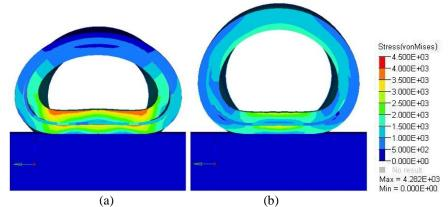
Figure 13. Comparison between tests at (a) 60MPa and (b) 600MPa of internal pressures.
