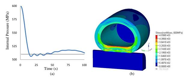
Figure 12. (a) Internal pressure and (b) von Mises stress at critical instant of the drop test.
