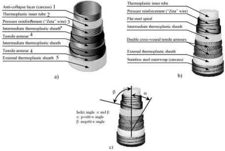
Figure 1. (a) and (b) Profiles Pattern Flexible Pipelines and (c) helix angle ( $\alpha$  and  $\beta$ ). Extracted from Dias et al. (1995).
