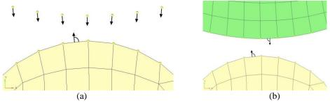
Figure 4. (a) Contact Nodes to Surface and (b) Contact Surface to Surface.
