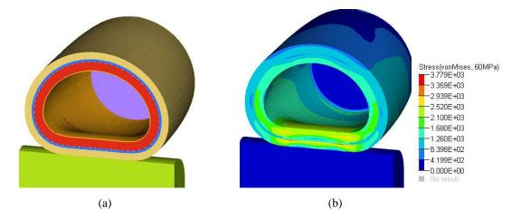
Figure 11. (a) Deformed profile of the riser and (b)Von Mises stress, for the drop test with internal pressure of 600MPa.
