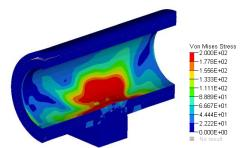
Figure 7. Stress in the riser during simulation of drop test.
