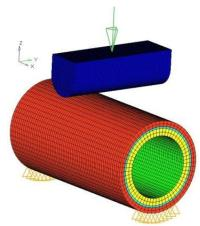
Figure 5. Model of the riser without internal pressure.
