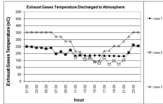
Fig. 15 – Exhaust gas temperature discharged to atmosphere (cases 1, 2 and 3)
