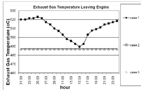
Fig. 13 – Engine exhaust gas temperature (cases 1 to 3)
