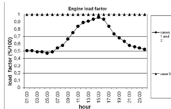
Fig. 9 – engine load factor (cases 1, 2 and 3)
