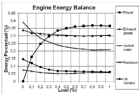
Figure 6 – Engine Energy Balance
