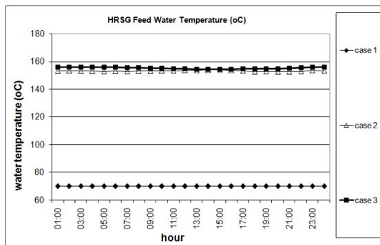
Fig. 14 – HRSG feed water temperature (cases 1 to 3)
