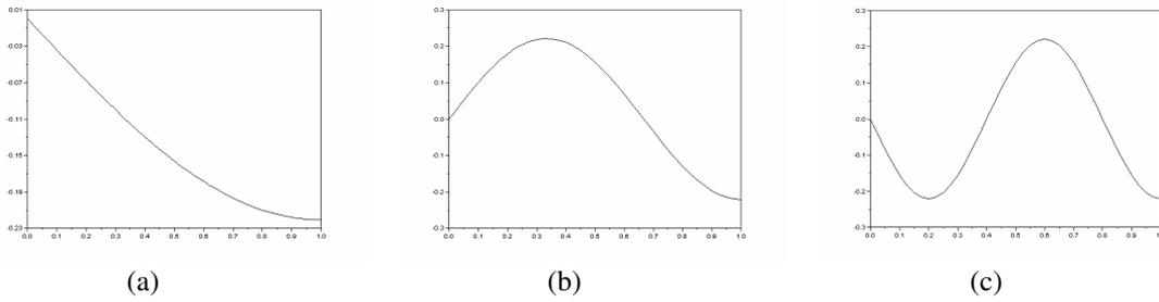
Figure 4. Longitudinal vibration: (a) mode 1, (b) mode 2 and (c) mode 3.
