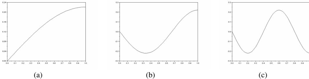
Figure 6. Torsional vibration: (a) mode 1, (b) mode 2 and (c) mode 3.
