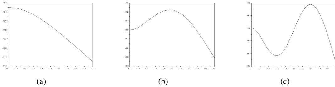
Figure 5. Transverse vibration: (a) mode 1, (b) mode 2 and (c) mode 3.
