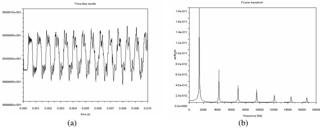
Figure 7. Longitudinal vibration using  $N = 2098$  and  $\Delta t = 10^{-5} s$ : (a) endpoint response and (b) corresponding FFT.
