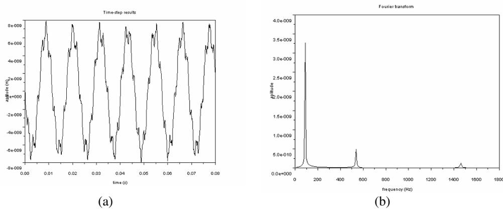
Figure 8. Transverse vibration using  $N = 2098$  and  $\Delta t = 5 \cdot 10^{-5} s$ : (a) endpoint response and (b) corresponding FFT.
