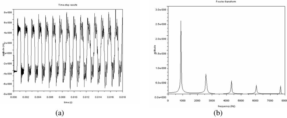
Figure 9. Torsional vibration using  $N = 2098$  and  $\Delta t = 10^{-5} s$ : (a) endpoint response and (b) corresponding FFT.
