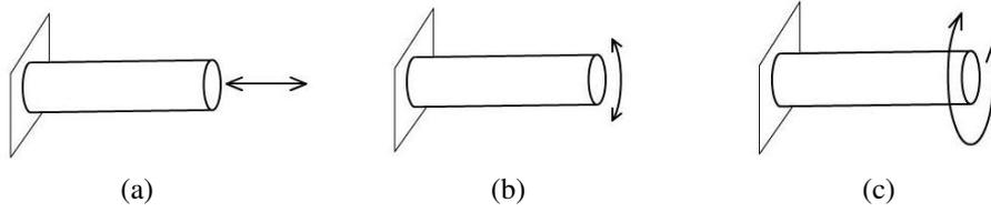
Figure 2. Cantilever beam and the three situations of vibration.
