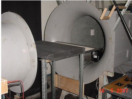
Figure 3. Cavity model in the wind tunnel.
