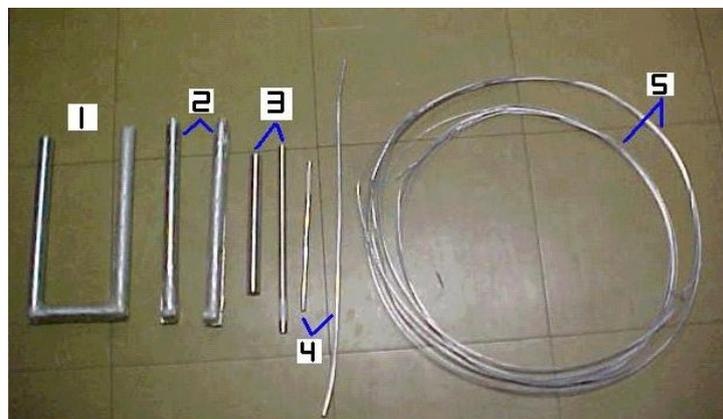
Figure 6 – Sequence of operational stages until diameter 3, 45 mm.
