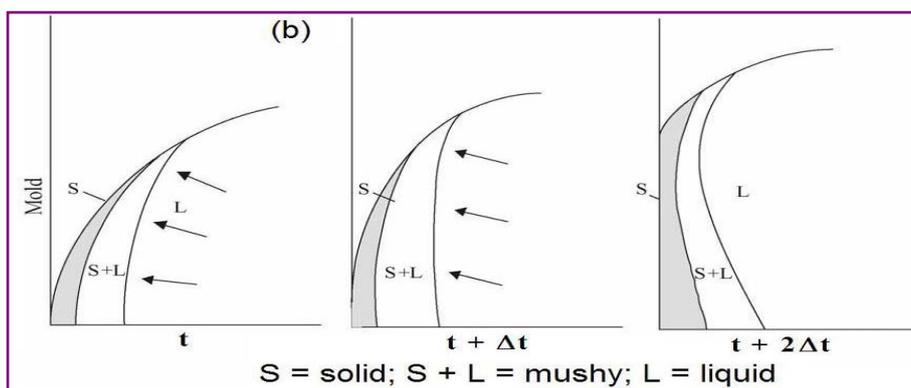
Figure 4 – Action Illustration of metal pressure and motive power during the alloys solidification with larger time solidification or high fluidity.
