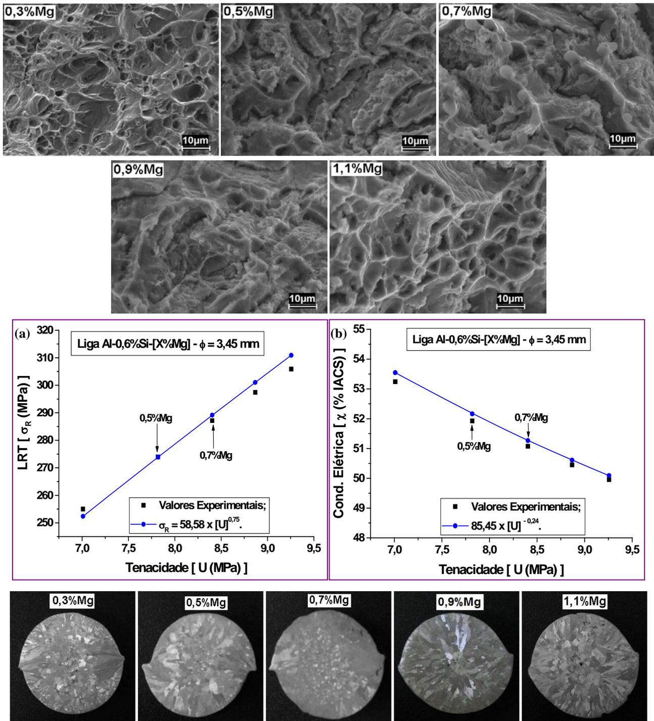
Figure 8 – LRT and Strength in relation to Mg content.
