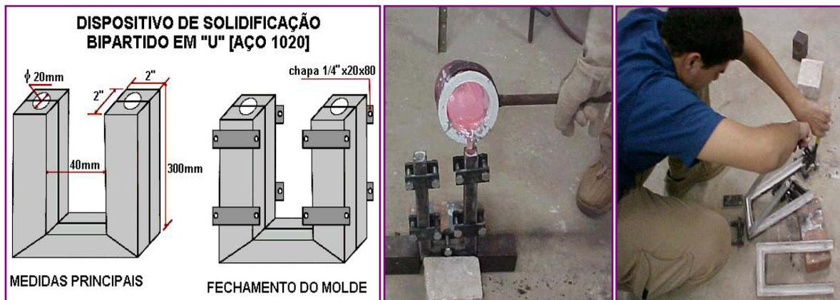
Figure 5 – Sequence of operations to obtaining the “U” specimen.
