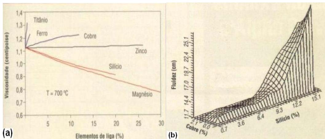
Figure 1 - Influence of alloy elements on aluminium viscosity, Verran, 2004 and on aluminum fluidity variation depending of silicon and copper content, Kim e Loper, 1995.
