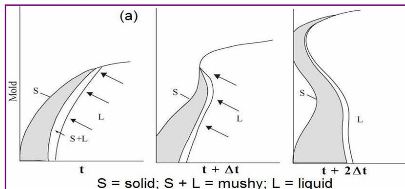
Figure 3 – Illustration of metal pressure and motive power during the alloy solidification with short time solidification or low fluidity.
