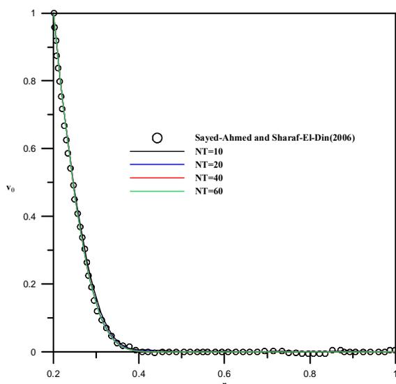
Figure 6. Velocity profile  $v_0$  for  $\gamma = 0.2$  at  $Z = 0.002$ .
