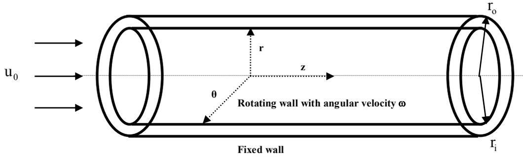
Figure 1. Geometry and coordinate system for developing annular flow with rotation of the inner wall.
