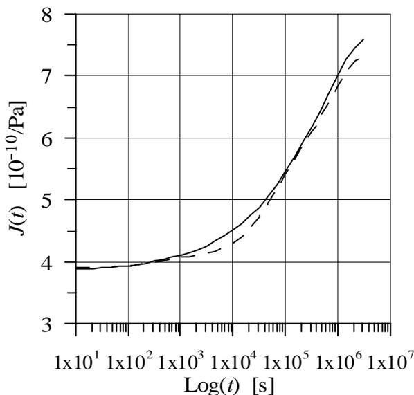
Figure 3. Diagrams for total creep modulus: continuous line obtained from experimental data and dashed line from recovered parameters of Table 5.
