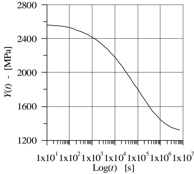
Figure 2. Diagram for total relaxation modulus of PVC, extracted from creep test.
