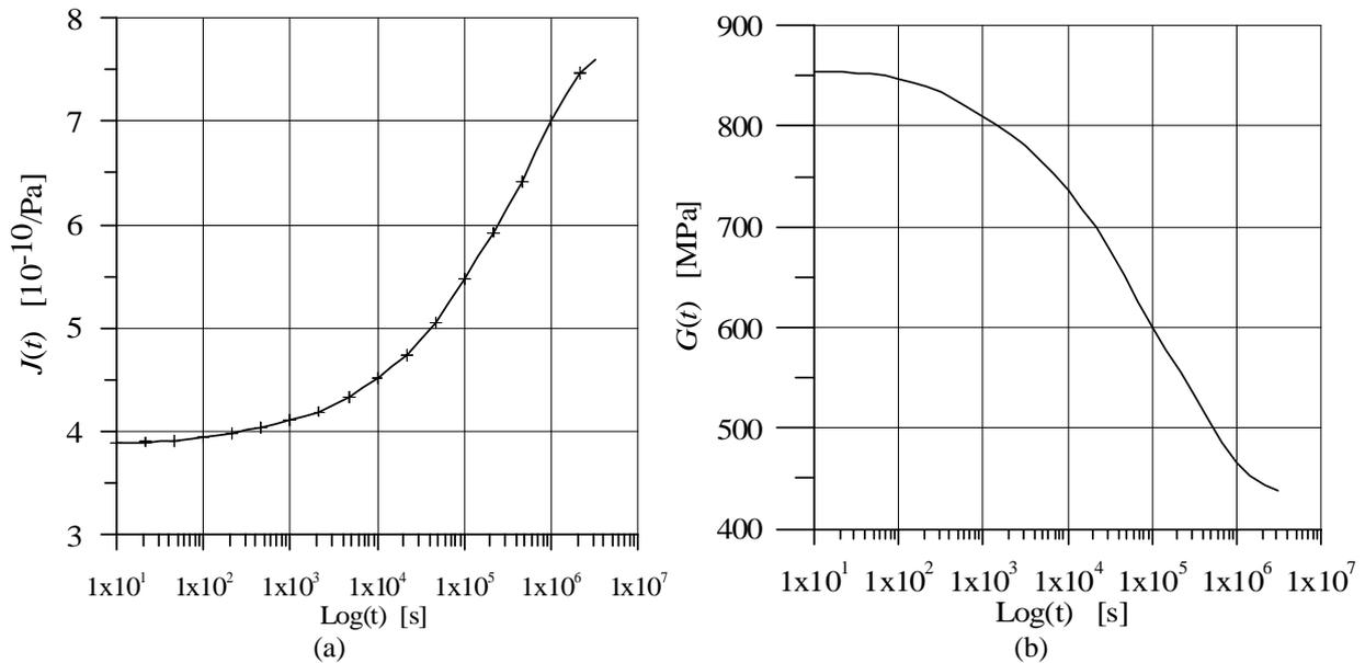
Figure 1. Diagrams for total creep modulus in (a) and for deviatoric relaxation modulus in (b).
