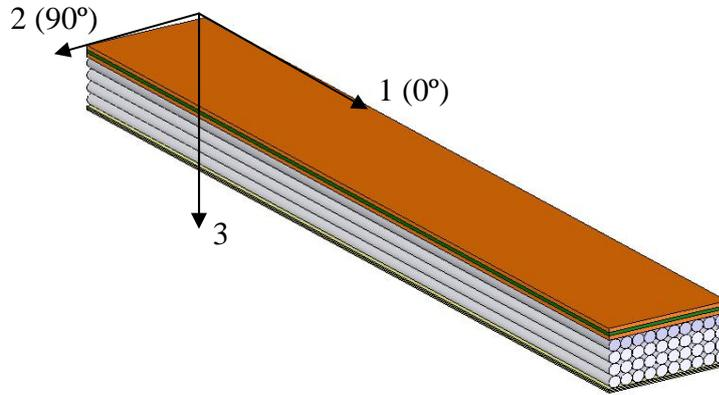
Figure 4. Composite beam with fibers parallel ( $0^\circ$ ) to axis 1.
