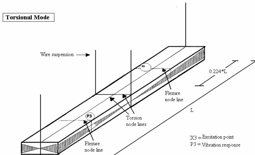
Figure 3. Supports, excitation and vibration response of torsional modes measurements.
