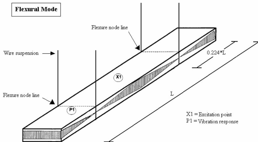
Figure 2. Supports, excitation and vibration response of flexural modes measurements.
