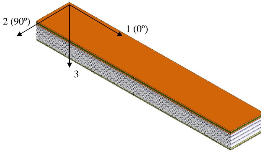
Figure 5. Composite beam with fibers perpendicular ( $90^\circ$ ) to axis 1.
