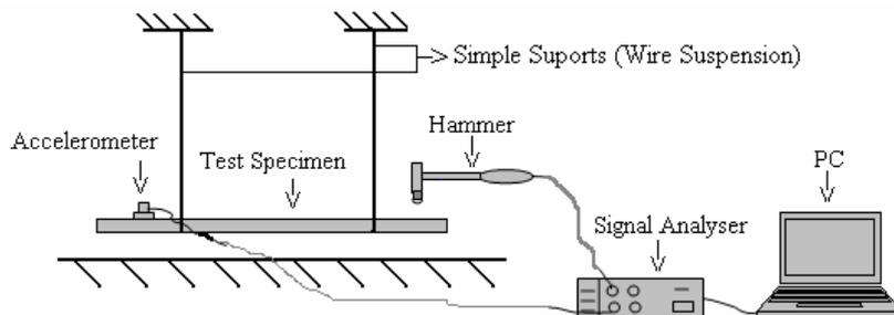
Figure 1. Apparatus for dynamic properties measurement.
