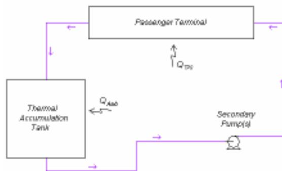
Figure 6. Simplified project of the operation with the use of thermal accumulation
