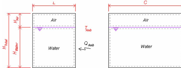
Figure 5. Volume of control for the second stage
