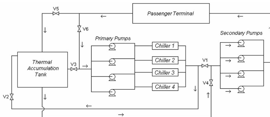
Figure 1. Thermal accumulation system of frozen water
