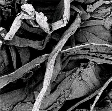
**Figure 12.** SEM micrograph bleached cellulose 500X secondary electrons.
