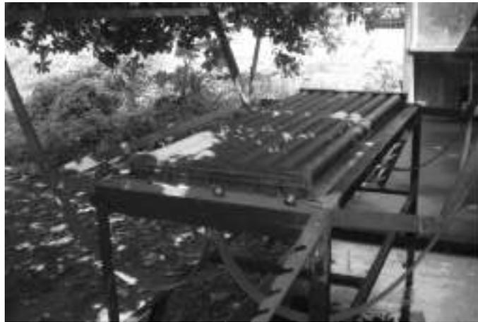
Figure 10. The view of CPC structure and the adsorber at the Laboratory of Solar Energy.
