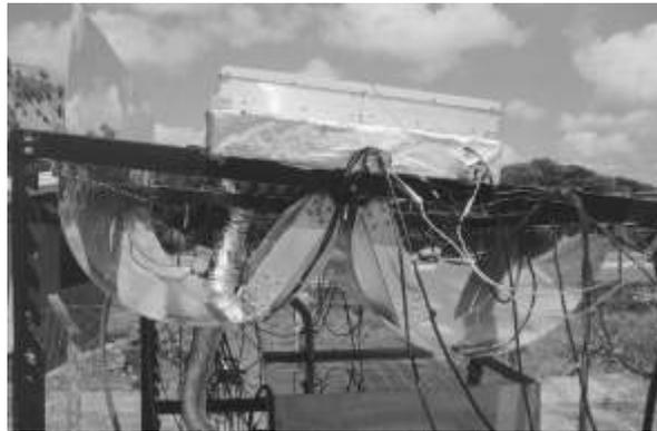
Figure 2. Lateral view of the collector, TIM covers and the concentrator.
