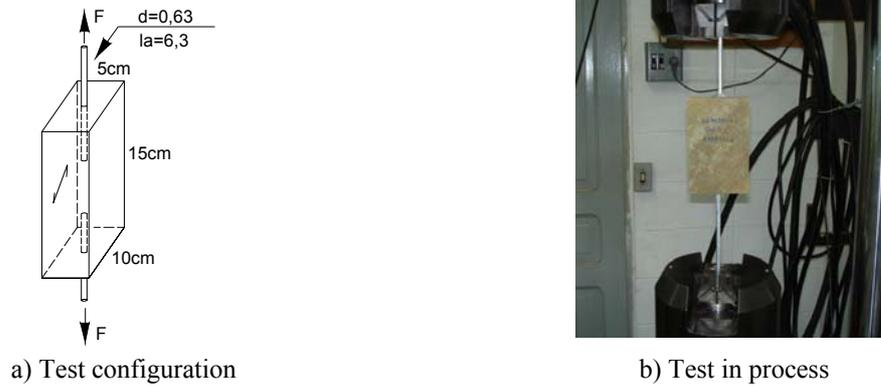
Figure 2. Fatigue and static tests
