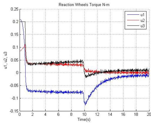
Figure 3 – Reaction wheels control torque histories.
