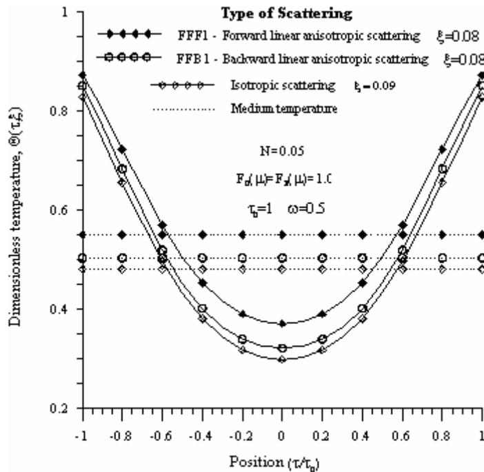
Figure 3: Effect of the scattering in the distribution of temperature in a ceramic body with constant thermal properties such as  $N = 0.05$ , Biot = 5 and external radiation sources  $F_0(\mu) = F_3(\mu) = 1$ .
