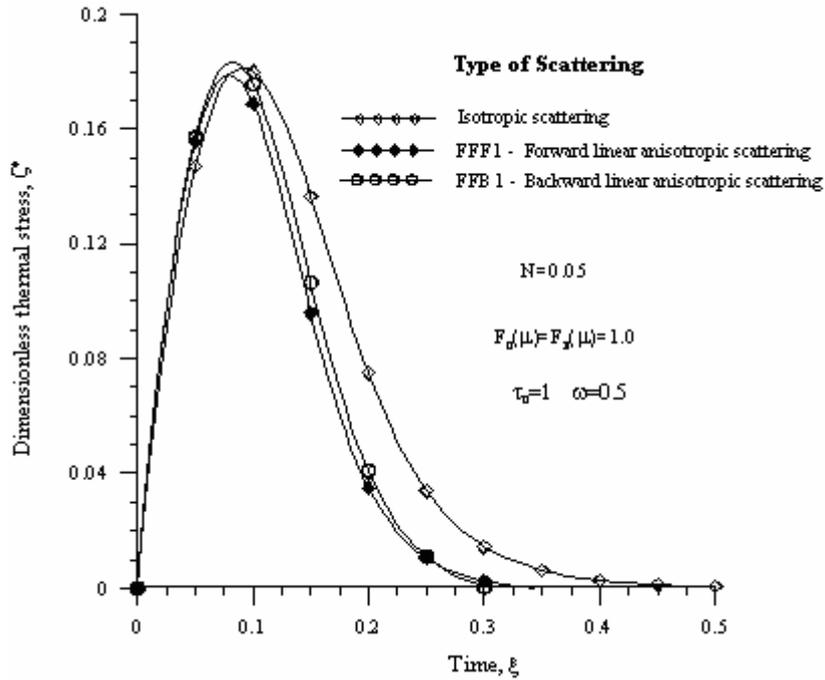
Figure 2- Effect due to the scattering of the thermal tensions in a ceramic body with constant thermal properties and  $N = 0.05$ , Biot number = 5 and external radiation  $F_0(\mu) = F_3(\mu) = 1.0$ .
