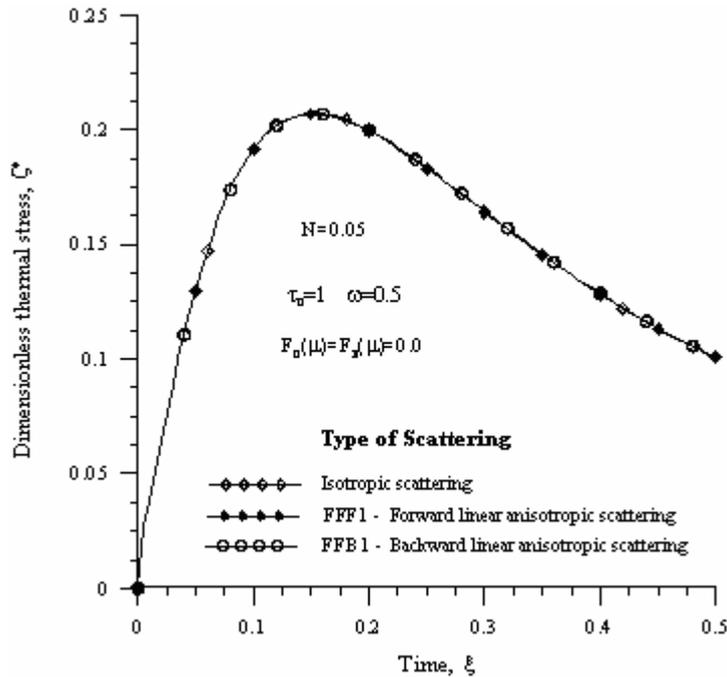
Figure 4: Effect of the scattering in the thermal tensions of a ceramic body with constant thermal properties such as  $N = 0.05$ , Biot = 5 and external radiation sources  $F_0(\mu) = F_3(\mu) = 0$ .
