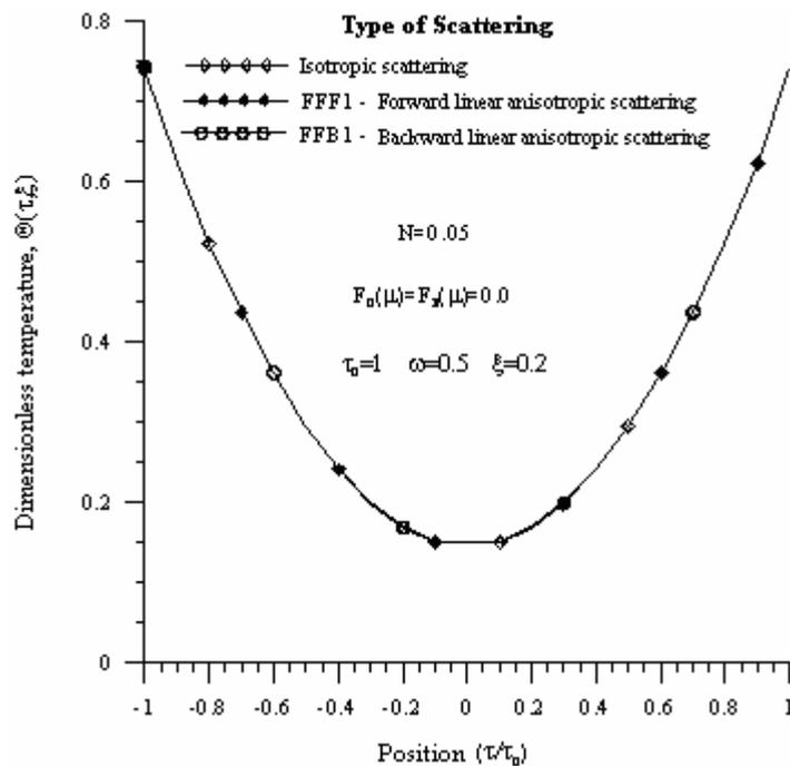
Figure 5: Effect of the scattering in the temperature distribution on a ceramic body with Constant thermal properties such as  $N = 0.05$ , Biot = 5 and external radiation sources  $F_0(\mu) = F_3(\mu) = 0$ .
