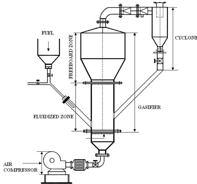
Figure 1: Schematically diagram of fluidized bed gasifier.
