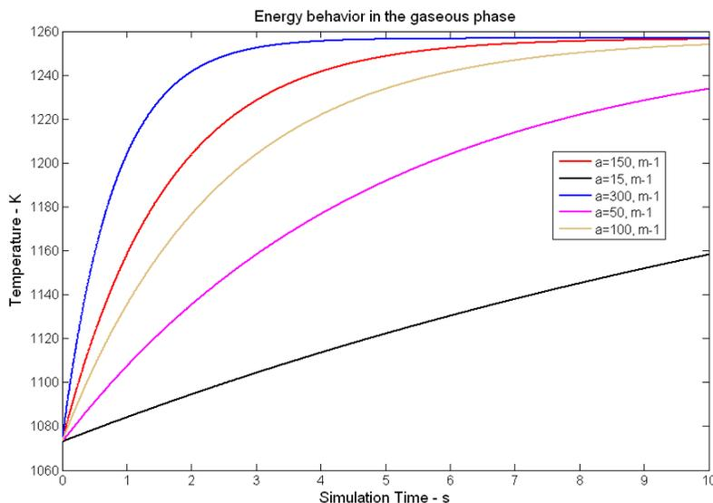
Figure 5: Temperatures profiles to the gaseous phase in several kinds of interfacial area.
