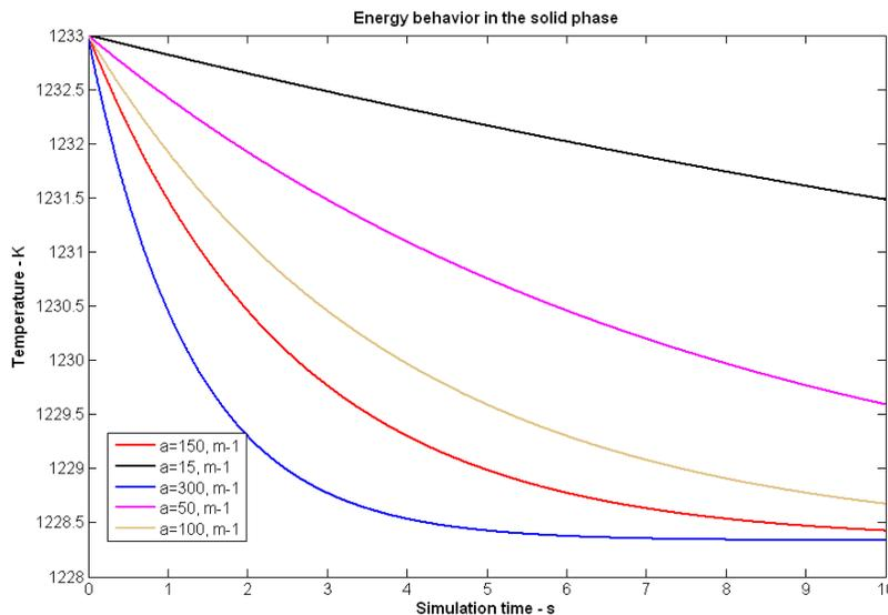
Figure 6: Temperatures profiles to the solid phase in several kinds of interfacial area.
