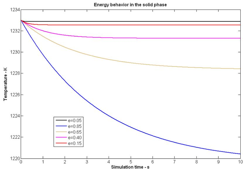
Figure 5: Temperature profile of several kinds of porosity in solid phase
