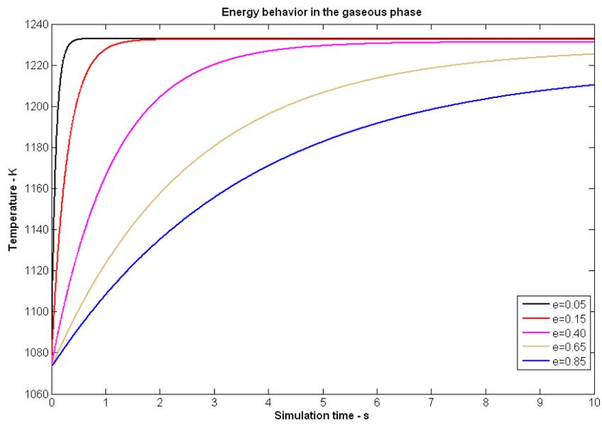
Figure 4: Temperature profiles of several kinds of porosity .in gaseous phase
