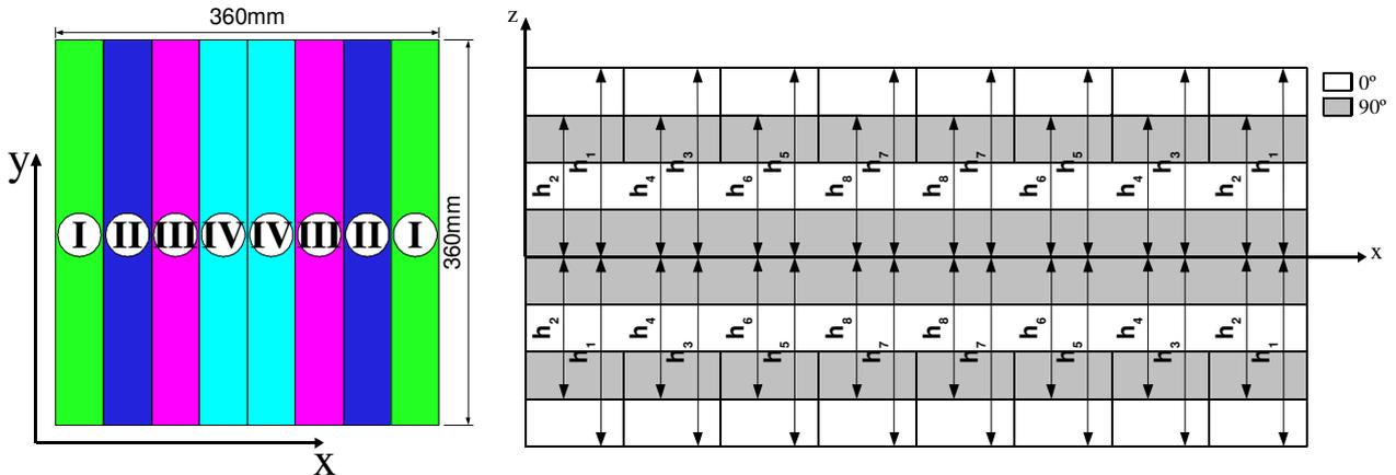
Figure 2. Geometry of plate with longitudinal reinforcements
