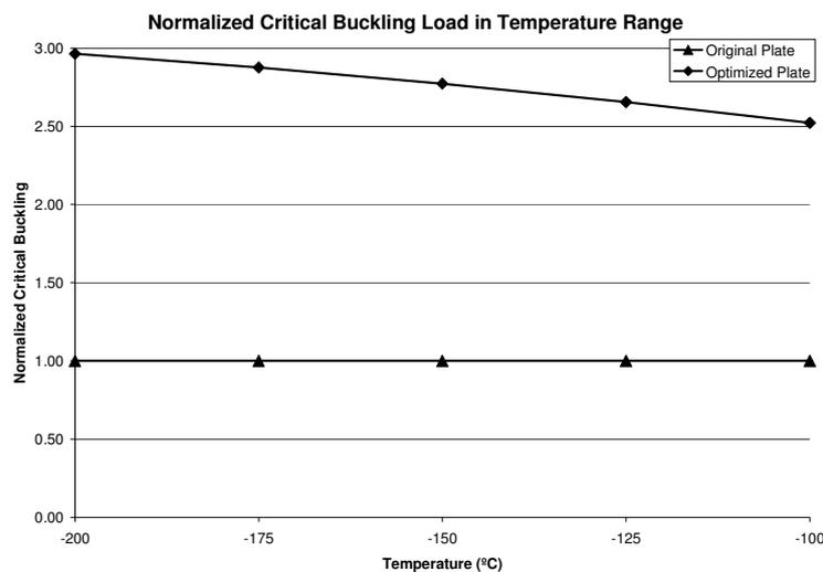
Figure 3. Case 1 normalized critical buckling load versus temperature
