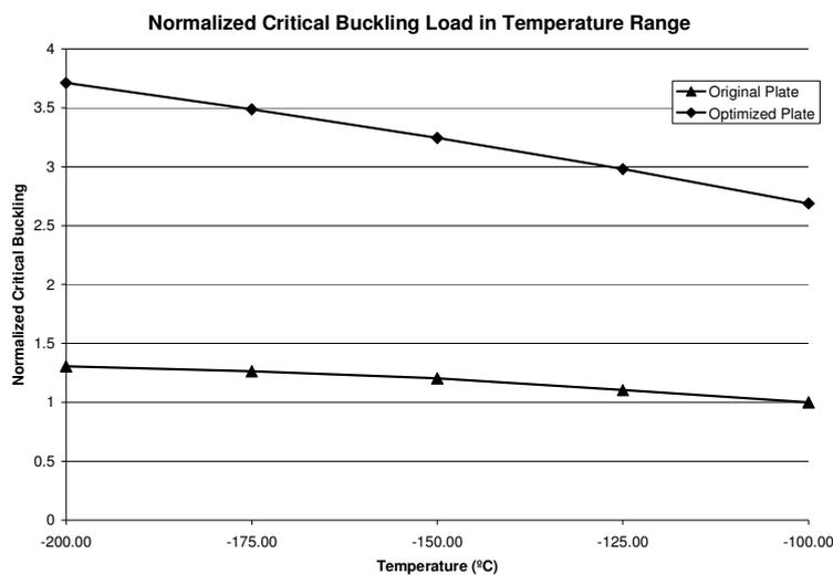
Figure 8. Case 2 normalized critical buckling load versus temperature
