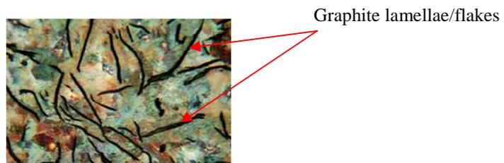
Figure 10 – SA 278 CL 40 micrograph
