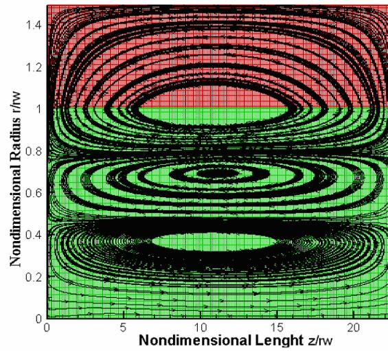
Figure 6. Streamlines for constant heat flux for rotation of 30,000 rpm
