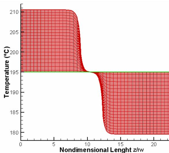
Figure 2. Temperature distribution for constant heat Flux for heat pipe operating at 5,000 rpm
