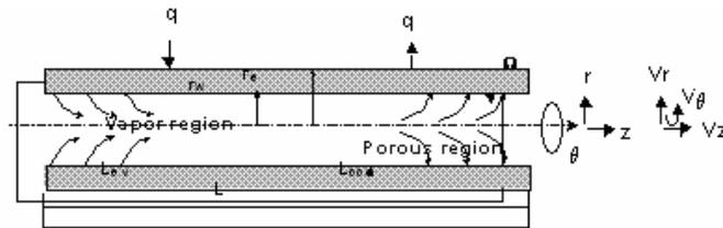
Figure 1. Schematic view of a rotating heat pipe.
