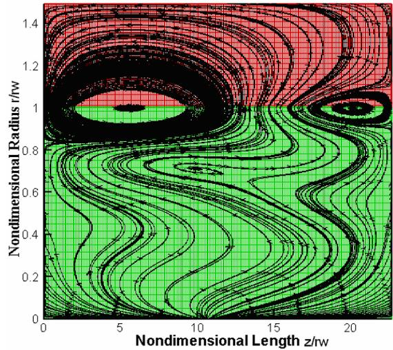
Figure 7. Streamlines profile for the given experimental temperature profile for rotation of 30,000 rpm
