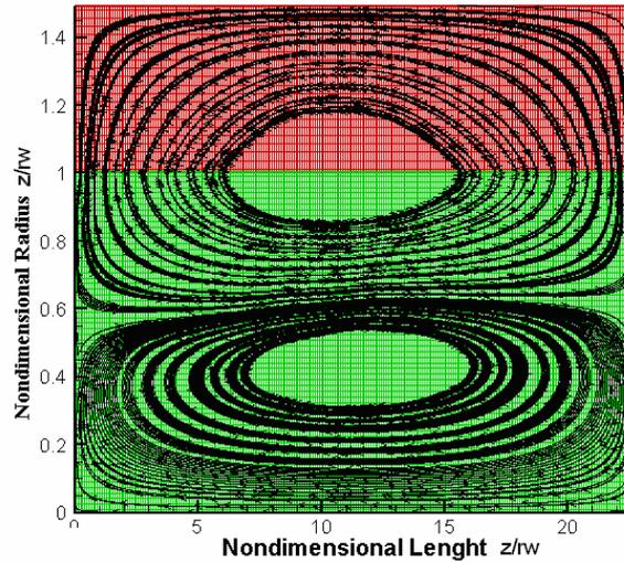
Figure 5. Streamlines for constant heat flux for rotation of 5,000 rpm
