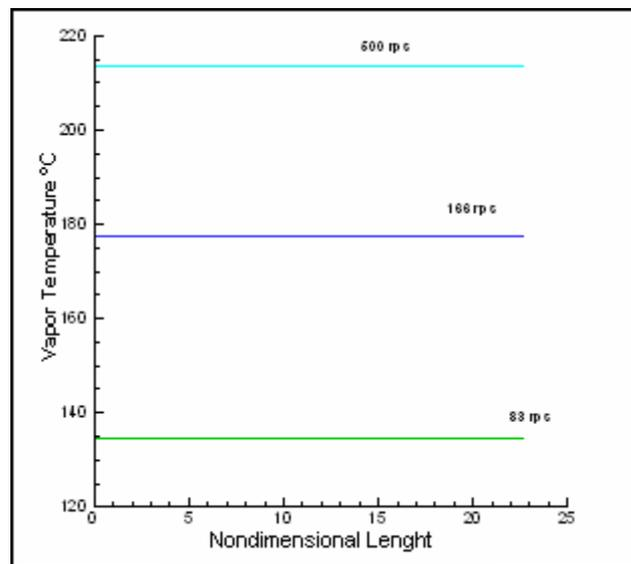
Figure 8. Saturation temperature for different heat pipe rotation.
