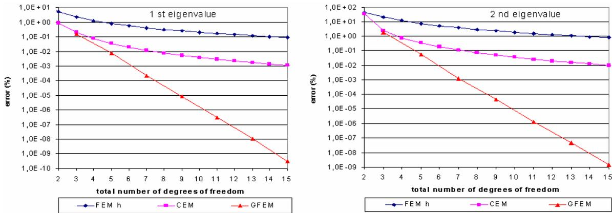
Figure 5. Relative error (%) for the 1st and 2nd bar eigenvalues.
