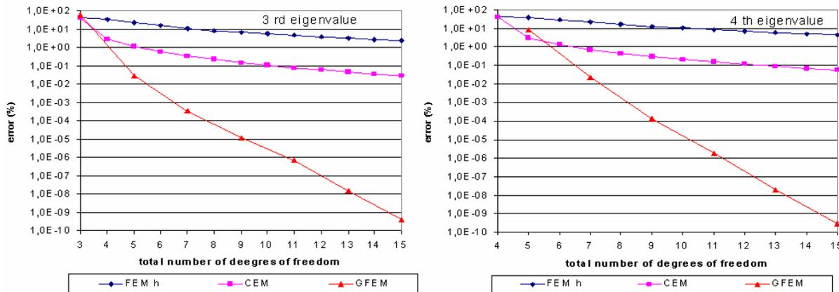
Figure 6. Relative error (%) for the 3rd and 4th bar eigenvalues.
