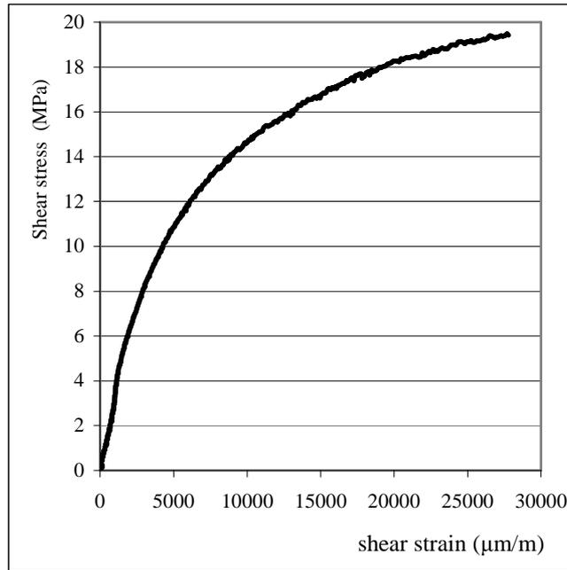
Figure 8. Shear strength for the as-cured samples
