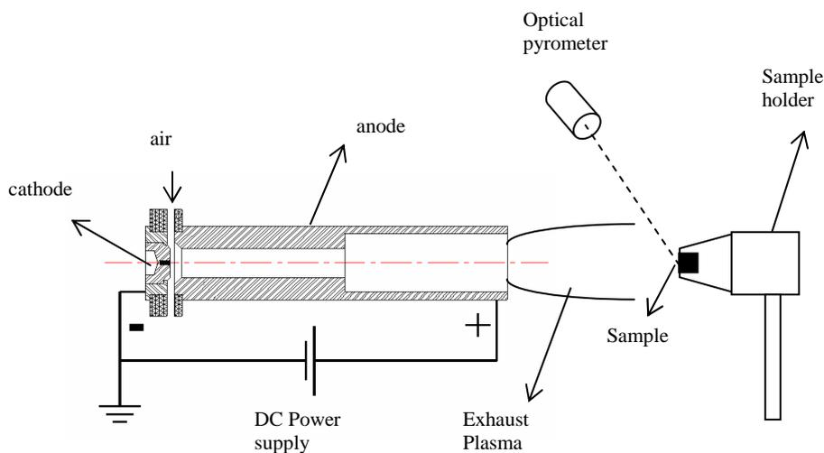
Figure 6. Schematic illustration of the apparatus for ablation test using an arc plasma torch
