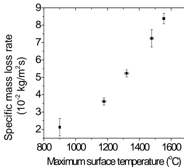
Figure 12. Specific mass loss rate as a function of maximum surface temperature
