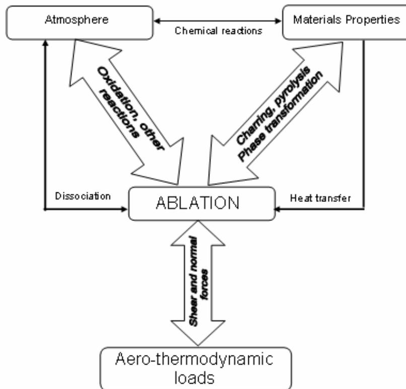
Figure 1. Schematic view of the influence of atmosphere, materials properties and aero-thermodynamic loads in the process of ablation
