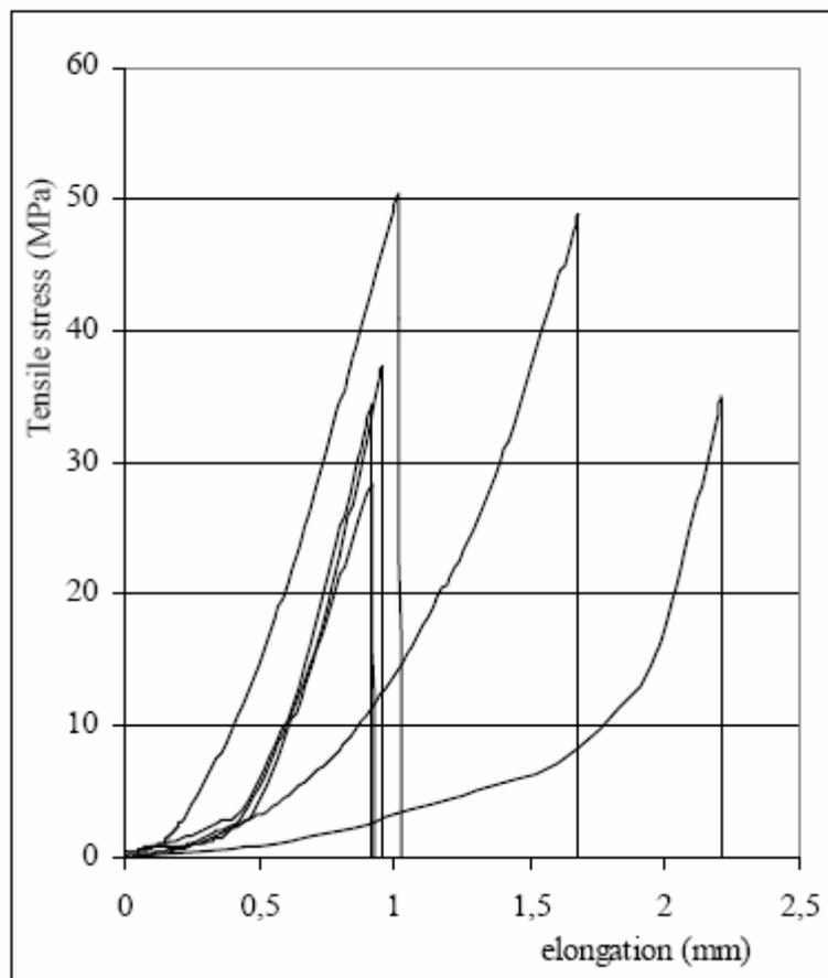
Figure 7. Tensile stress as a function of elongation for plain weave quartz phenolic composite
