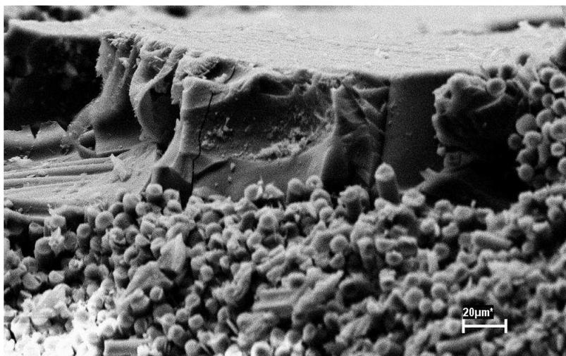
Figure 13. Surface of the quartz phenolic composite after the plasma torch burning test
