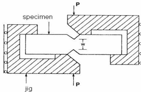
Figure 3. Scheme of the Iosipescu test jig
