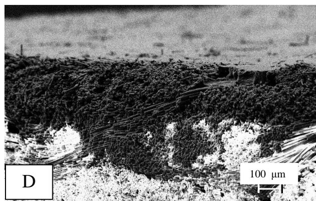
Figure 14. Side view of the specimens submitted to the plasma torch burning test
