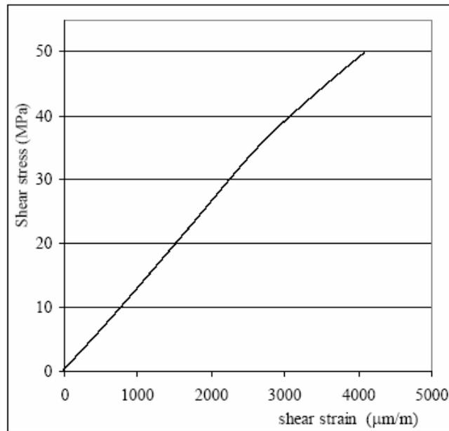
Figure 9. Shear strength for post-cured samples
