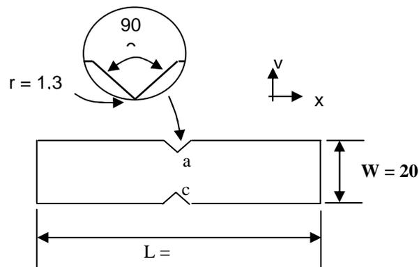
Figure 4. Specimen geometry used in Iosipescu test
