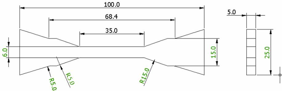
Figure 2. Geometry of test specimen for quartz phenolic composite
