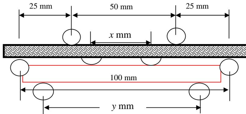
Figure 5. Sample geometry for flexural test
