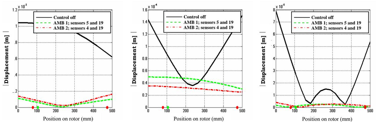
Figure 6. Local vibration along of rotor at critical frequencies of 19.2, 30.4 and 121.6 Hz, case E
