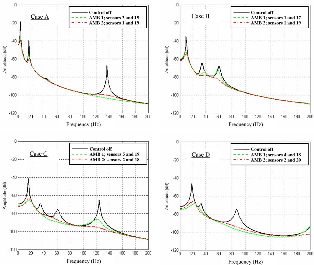
Figure 4. Global vibration reduction using control system with single actuator and two error sensors
