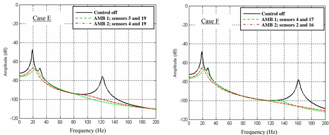
Figure 4. Global vibration reduction using control system with single actuator and two error sensors (Cont.)
