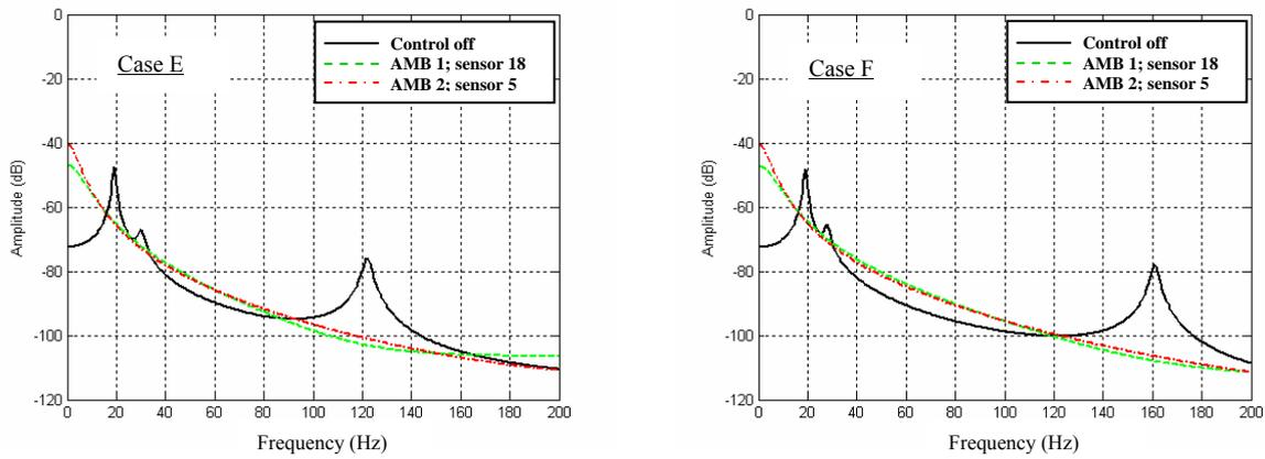
Figure 3. Global vibration reduction using control system with single actuator and single error sensor (Cont.)
