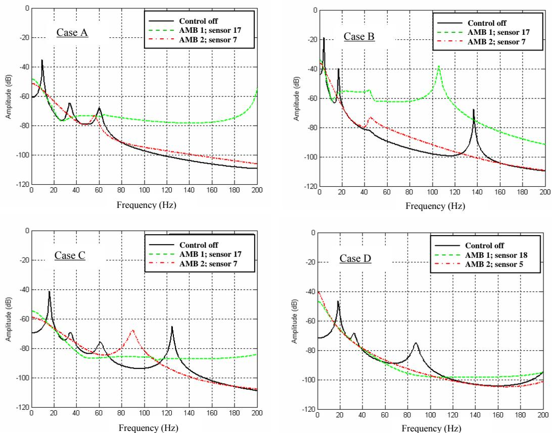
Figure 3. Global vibration reduction using control system with single actuator and single error sensor
