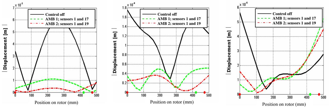
Figure 5. Local vibration along of rotor at critical frequencies 9.6, 33.6 and 48 Hz, case B
