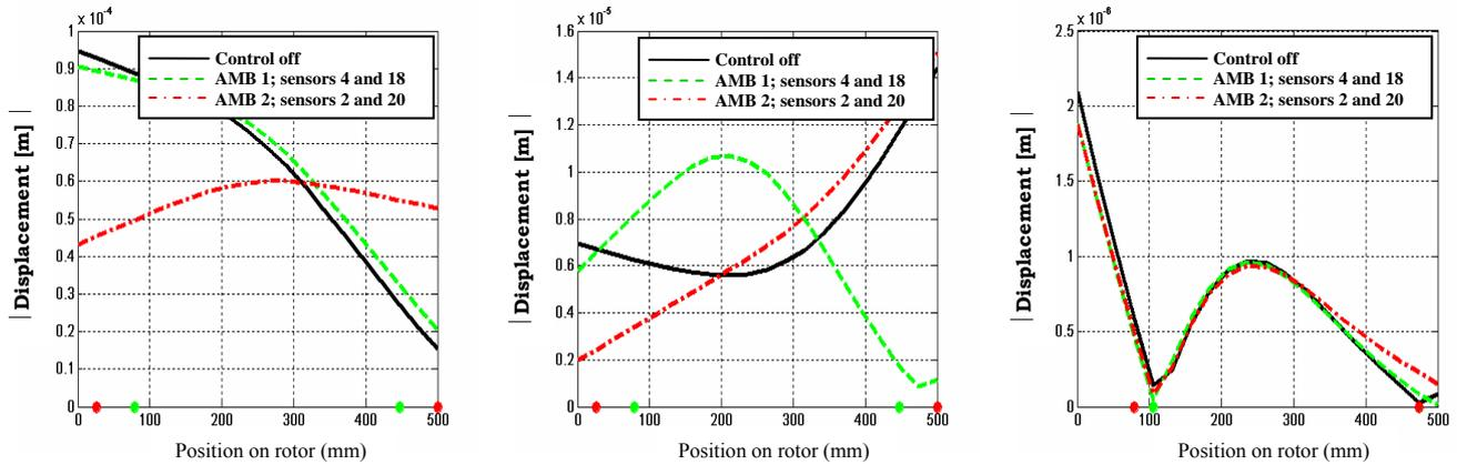
Figure 8. Local vibration along of rotor at frequencies 25.6, 60 and 160 Hz, case D
