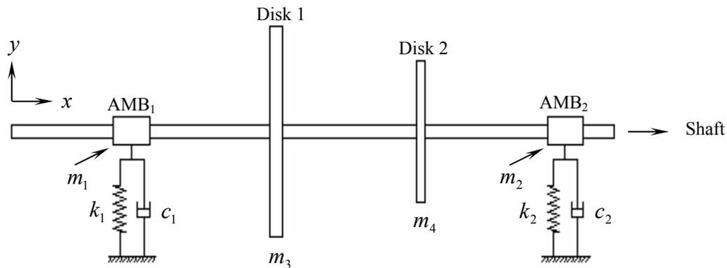
Figure 1. Schematic of rotor system used in theoretical model
