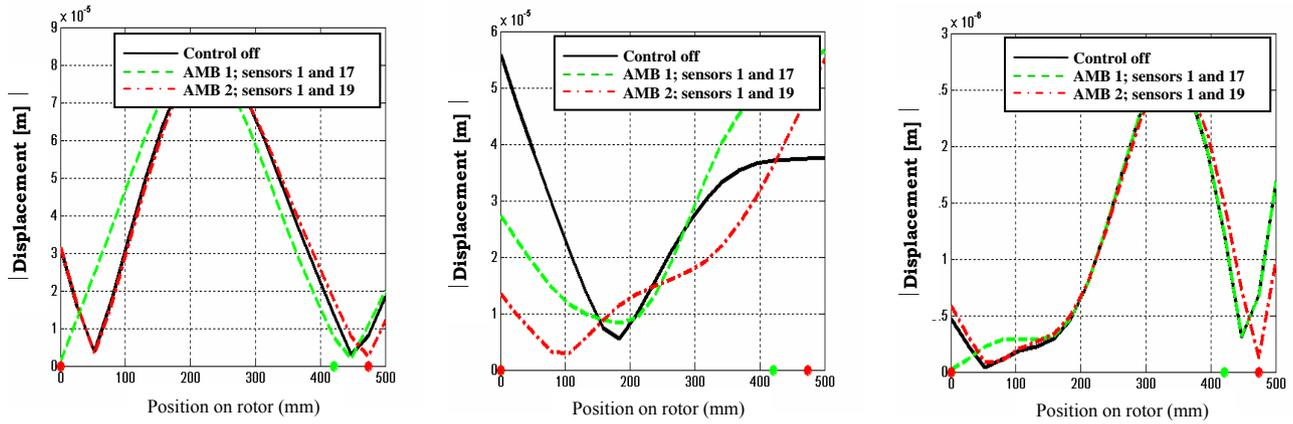
Figure 7. Local vibration along of rotor at frequencies 21.6, 40.8 and 140 Hz, case B
