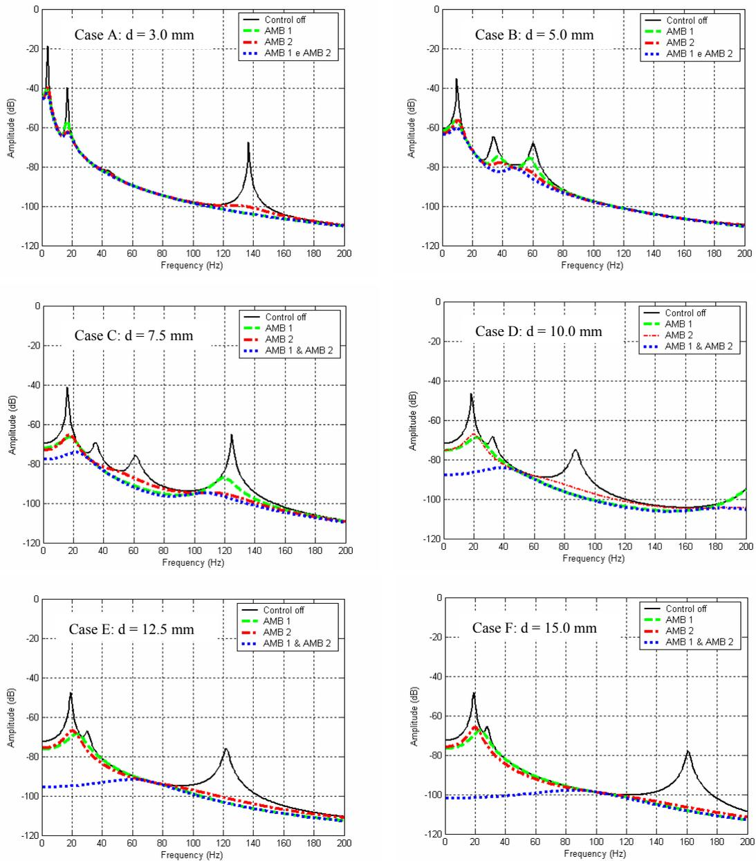
Figure 2. Global vibration reduction using the actuator 1, actuator 2 and both actuators, cases A to F.
