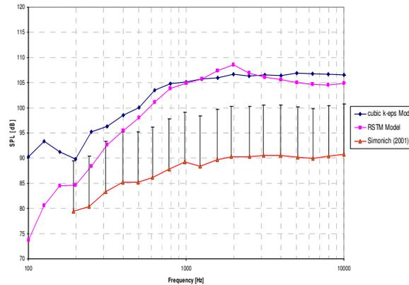
**Figure 14.** Turbulence modeling influence on the SPL.
