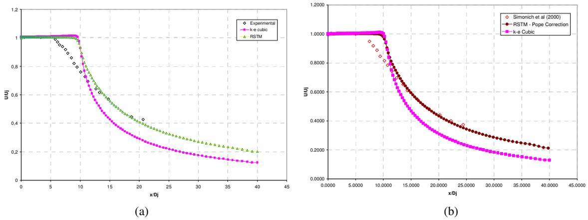
**Figure 6.** Jet centerline velocity distribution. (a) Mach = 0.6; (b) Mach = 0.9
