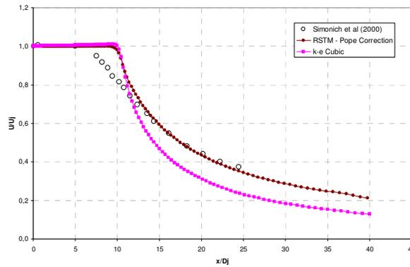
Figure 4. Turbulence influence in the axial velocity profile.
