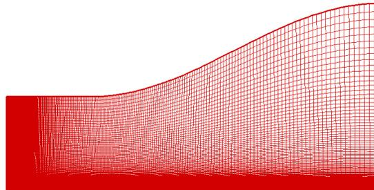
**Figure 2.** Computational 2D RANS mesh resolution (35000 cells).
