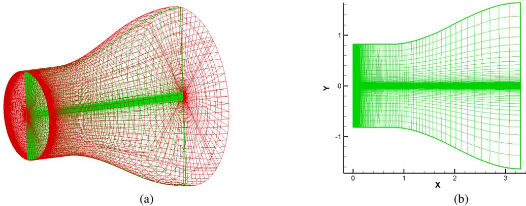
**Figure 3.** (a) Three-dimensional computational domain. (b) 3D computational slice.
