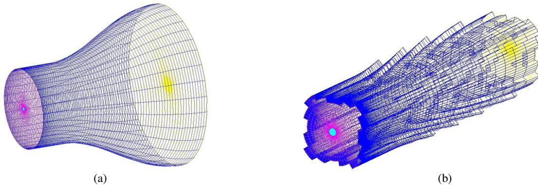
**Figure 5.** 3D Acoustics Meshes. (a) 310.000 cells. (b) 460.000 cells.
