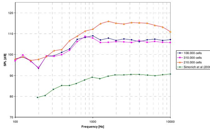
**Figure 9.** Acoustic Grid Independence Study.
