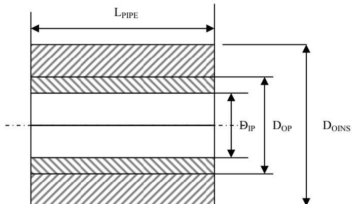
Figure 3 - Carbon steel pipe and its insulation
