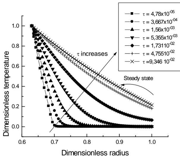
Figure 7. Temperature profiles in tube and insulation for each instant
