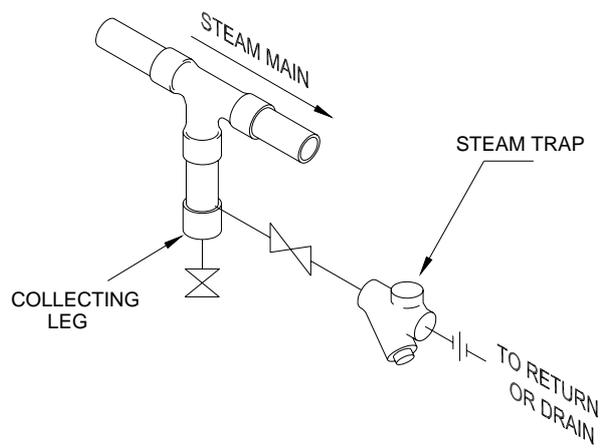
Figure 1. Collecting leg and steam trap on horizontal steam main
