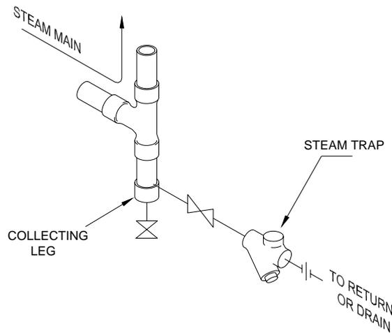
Figure 2. Collecting leg and steam trap on vertical steam main
