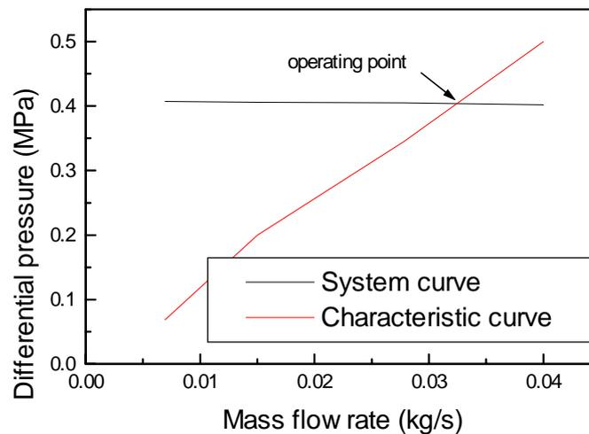
Figure 6. System and steam trap characteristic curves
