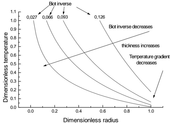
Figure 9. Steady state temperature profiles
