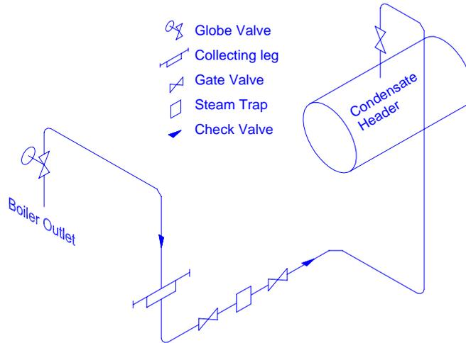
Figure 5. Layout of steam and condensate piping
