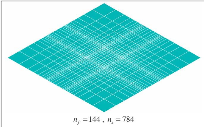
Figure 3: Half-space mesh for surface foundation
