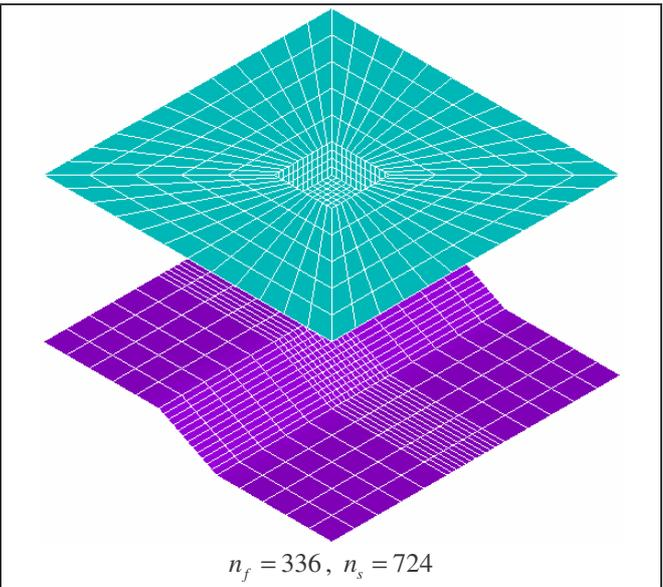
Figure 16: BE mesh for embedded foundation in a non-horizontal soil layer.
