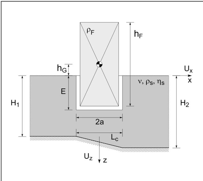
Figure 15: Scheme for foundation interacting with a non-horizontal soil layer.
