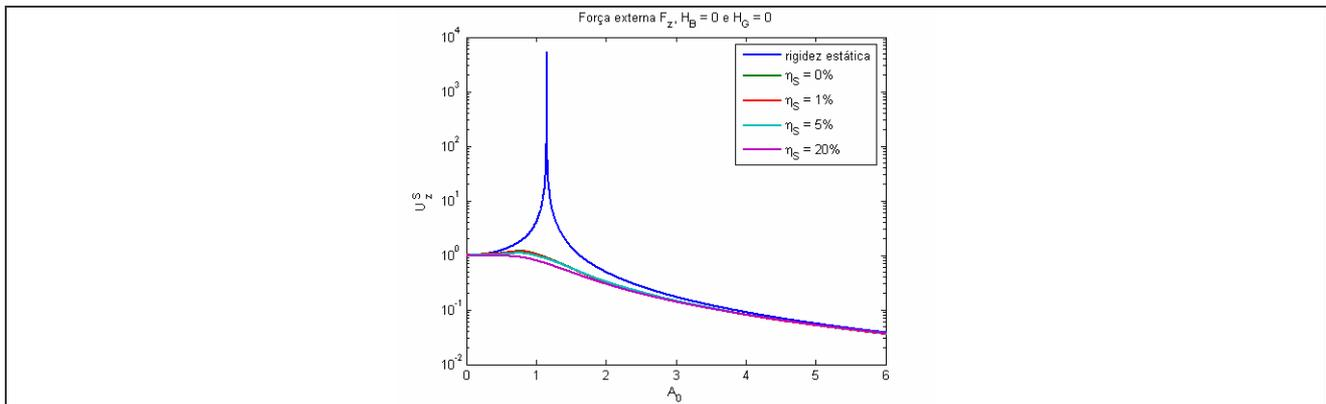
Figure 18: Vertical response of a block foundation over half-space considering distinct damping mechanisms
