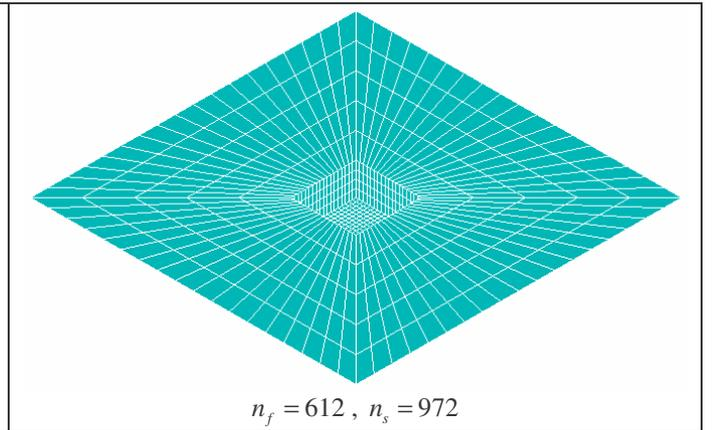
Figure 4: Half-space mesh for embedded foundation
