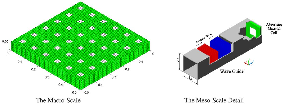
Figure 1. Insulation panel in macro scale modeling
