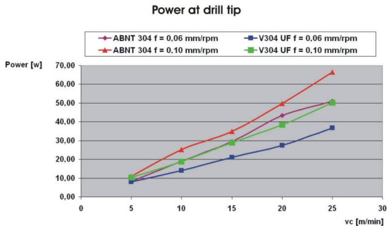
Figure 4 - Net power at drill tip
