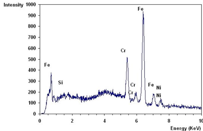
Figure 8 - EDS analysis of adhering layer that covers the main cutting edge.
