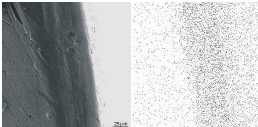
Figure 9 - WDS analysis of the drill main cutting edge.
