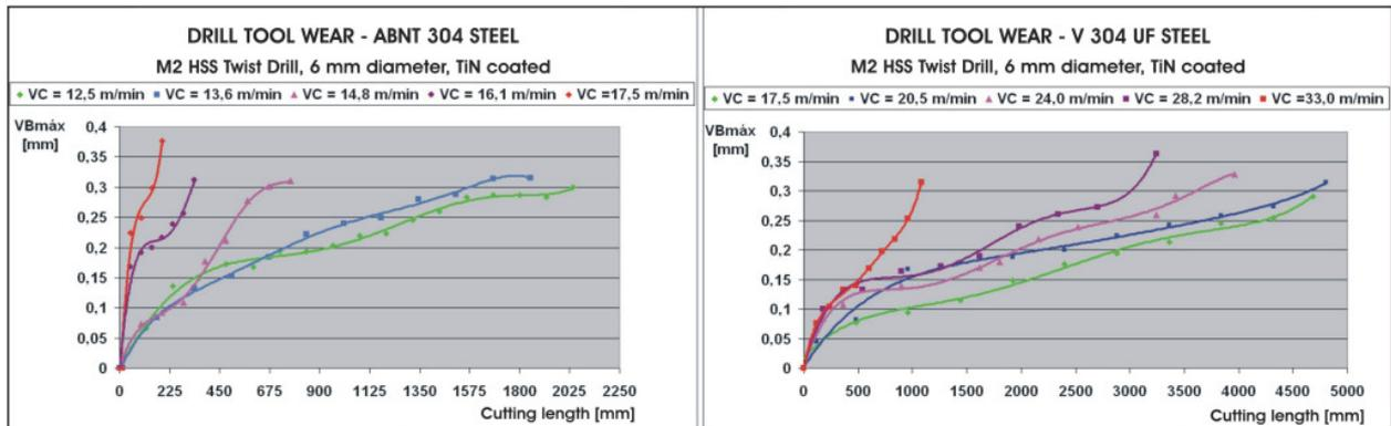
Figure 5 - Influence of workpiece material and cutting speed in hss twist drill tool wear
