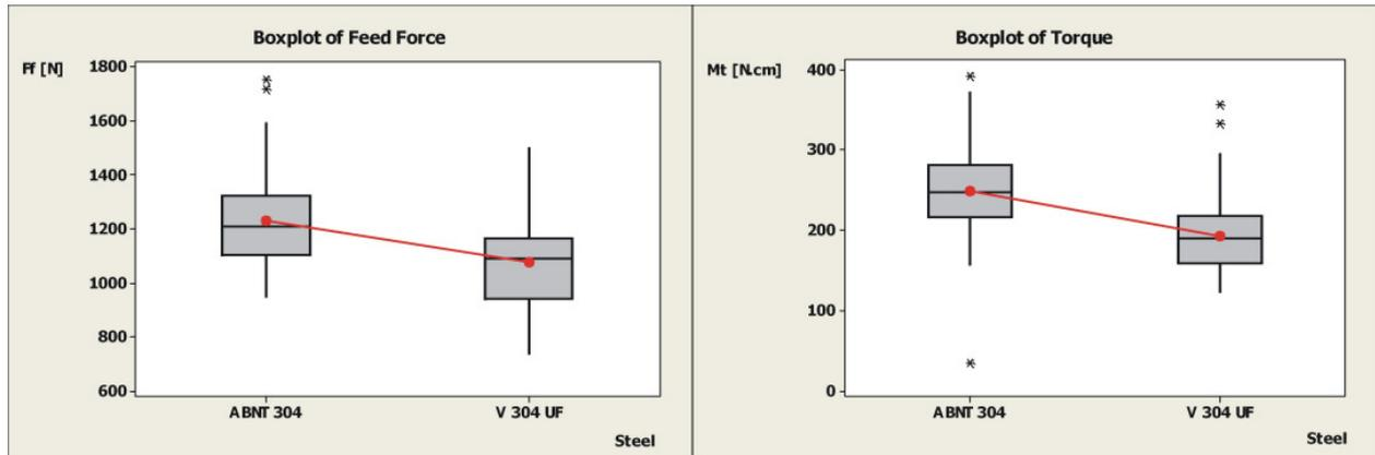
Figure 3 – Differences in feed force and torque with two austenitic stainless steels.
