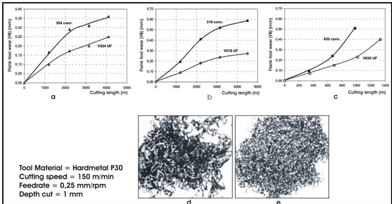
Figure 1 – Tool wear rates in turning a) V304 UF and ABNT 304 stainless steel b) V316 UF and ABNT 316 stainless steel c) V630 UF and ABNT 630 stainless steel. d) ABNT 304 chips e) V 304 UF chips.
