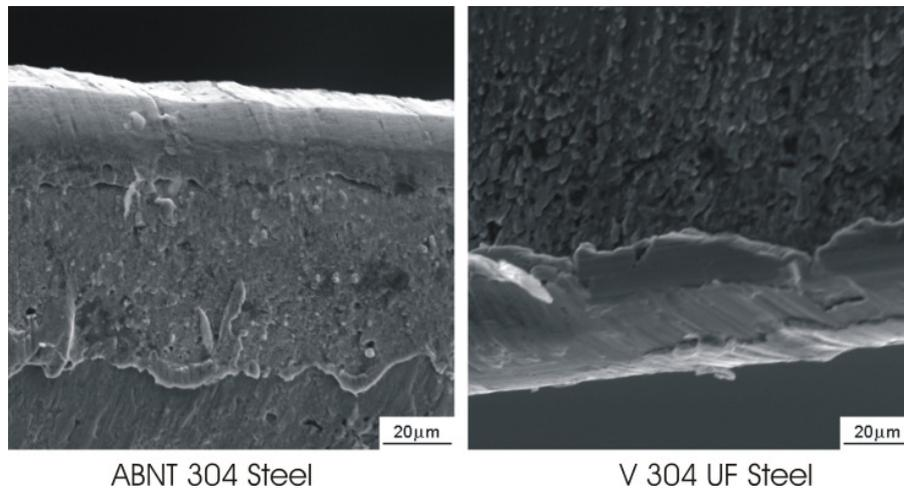
Figure 7 - Adhering layers that cover the main cutting edge.
