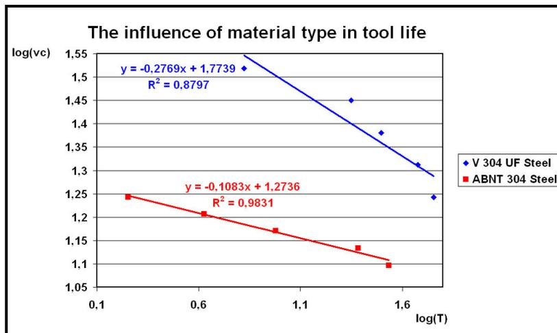
Figure 6 - Influence of workpiece material in drill tool life
