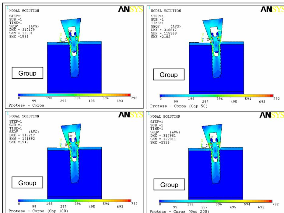
Figure 4: General stresses maps of the prosthesis/implant/retention screw system for groups 1, 2, 3, and 4.
