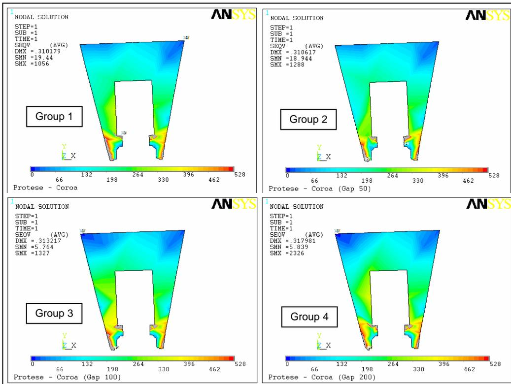
Figure 6: Plotted maps of the von Mises stresses distribution in the prosthesis in groups 1, 2, 3 and 4.
