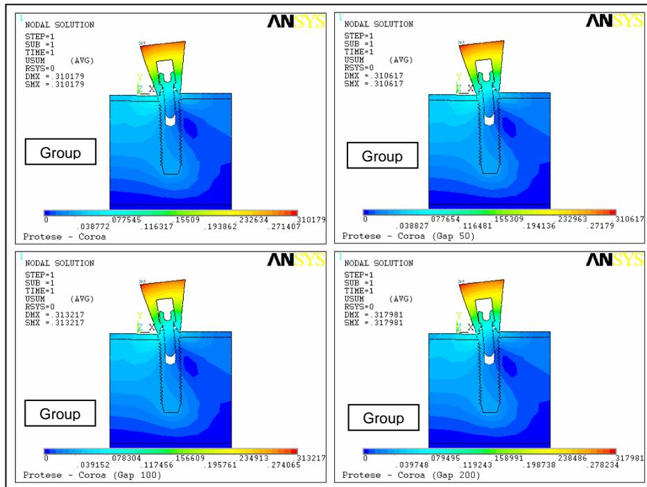
Figure 3: General maps of displacement conditions of the prosthesis/implant/retention screw system for groups 1, 2, 3, and 4.
