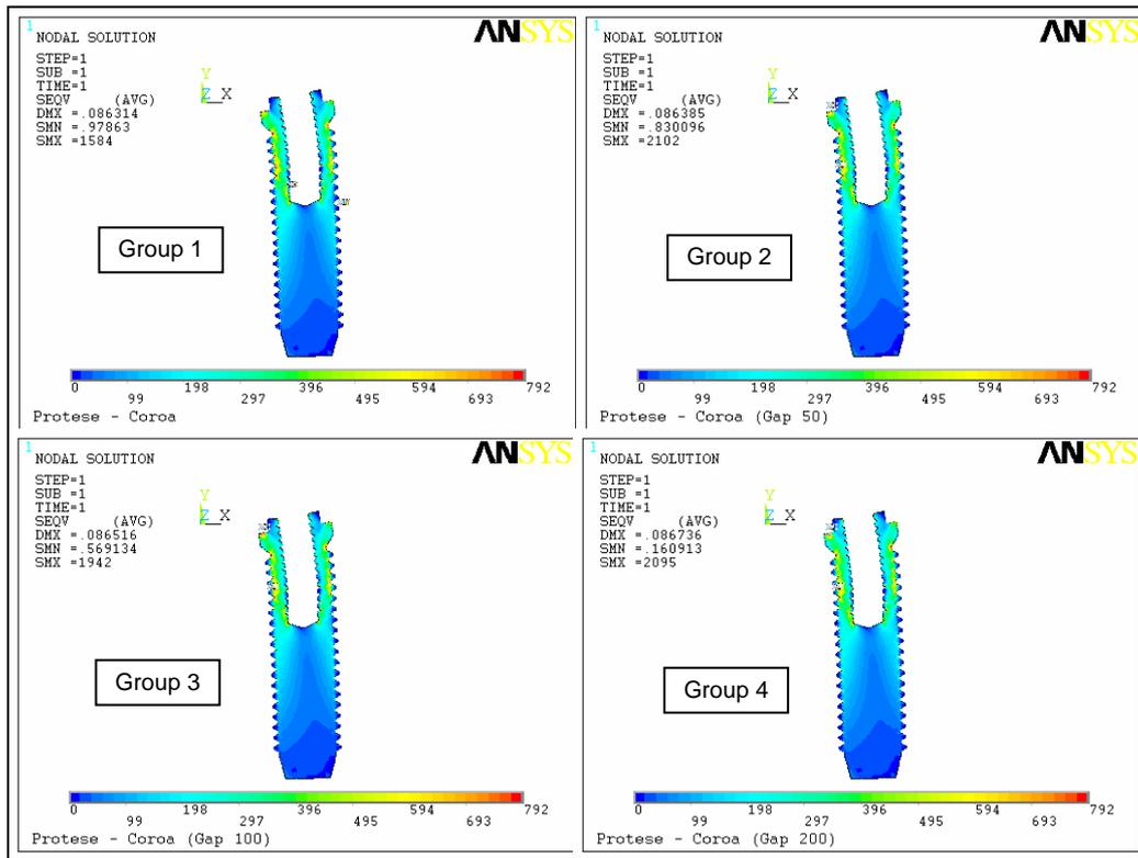
Figure 7: Plotted maps of the von Mises stresses distribution in the implant in groups 1, 2, 3 and 4.
