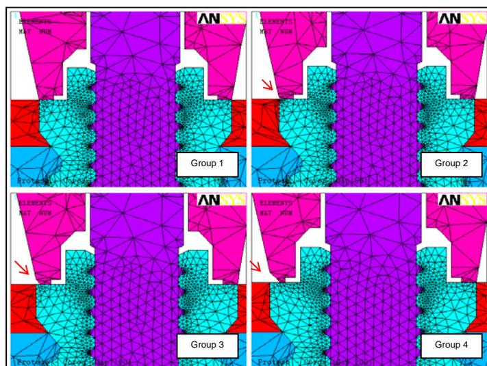
Figure 2: Approximate view of mesh elements in the region of contact between the prosthesis and the implant of groups 1, 2, 3 and 4, representing accurate fit and unilateral angular gaps of 50 $\mu$ m, 100 $\mu$ m and 200 $\mu$ m between the prosthesis and the implant, respectively.
