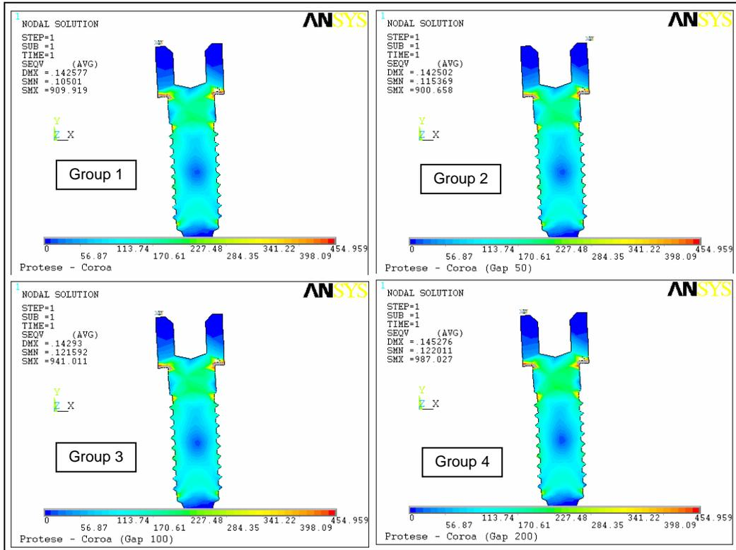
Figure 5: Plotted maps of the von Mises stresses distribution in the retention screw in groups 1, 2, 3 and 4.
