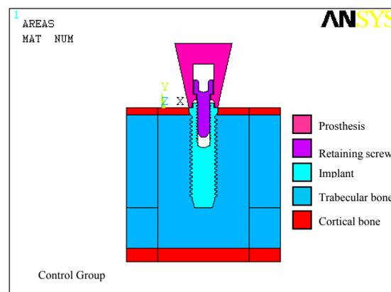
Figure 1: Model created in the finite element software representing prosthesis/implant/retention screw system in trabecular and cortical bone.
