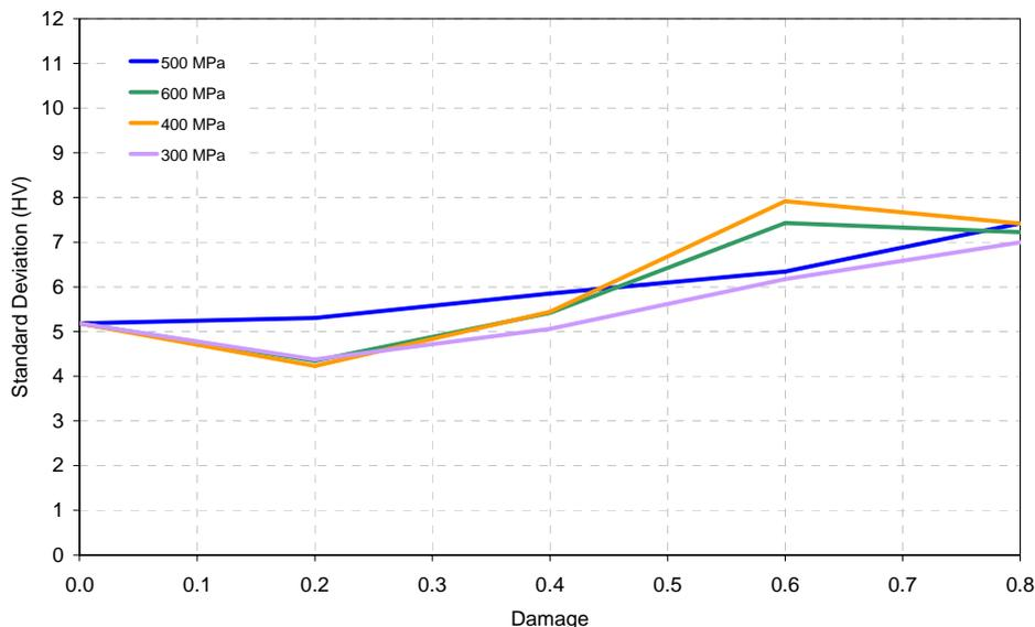
Figure 8 – Hardness standard deviation for the fatigue damaged specimens
