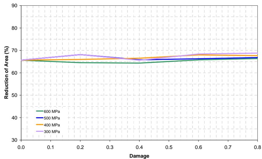
Figure 6 – Tensile test results – Reduction of Area
