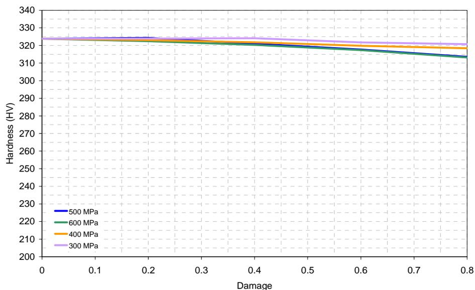
Figure 7 – Hardness average values for the fatigue damaged specimens
