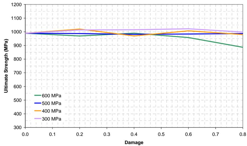
Figure 5 – Tensile test results – Ultimate Strength
