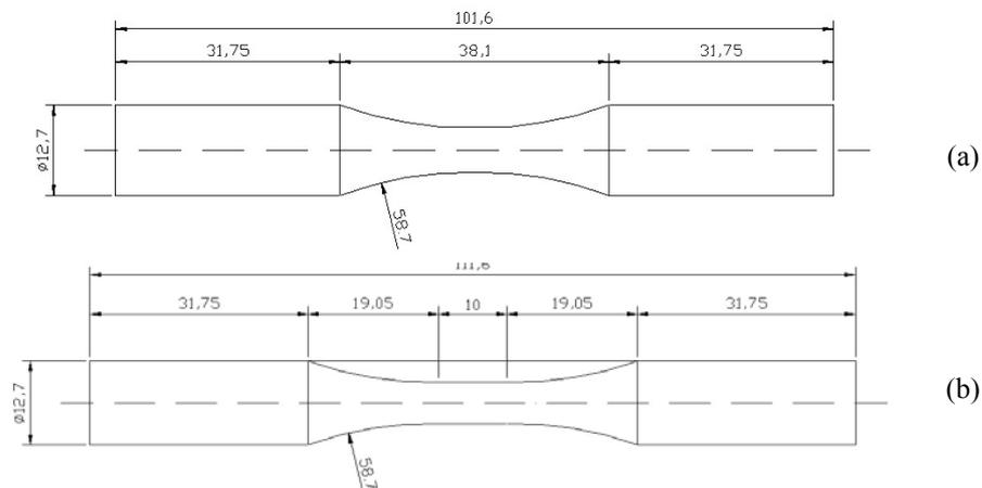
Figure 1 – Fatigue test specimen. (a) ASTM E466-96; (b) Modified for tests. Dimension in mm.
