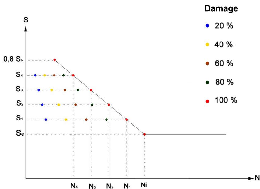
Figure 3 – Fatigue damage design based on the generated S-N curve
