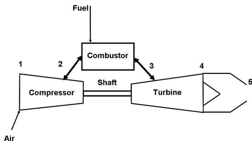
Figure 1. Turbine components diagram
