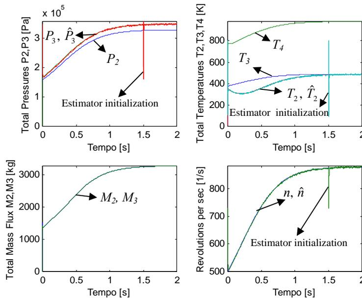
Figure 2. Performance of the EKF observer without control
