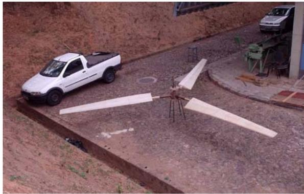
Figure 7. Rotor blades and hub of the *CEA WT-01* wind turbine
