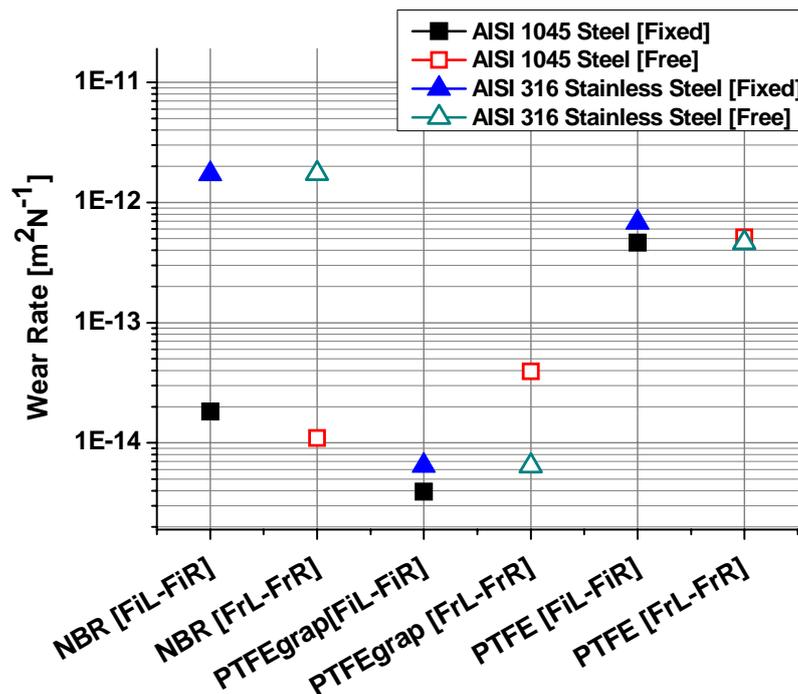
Figure 7. Wear rate from polymeric coupons after tests
