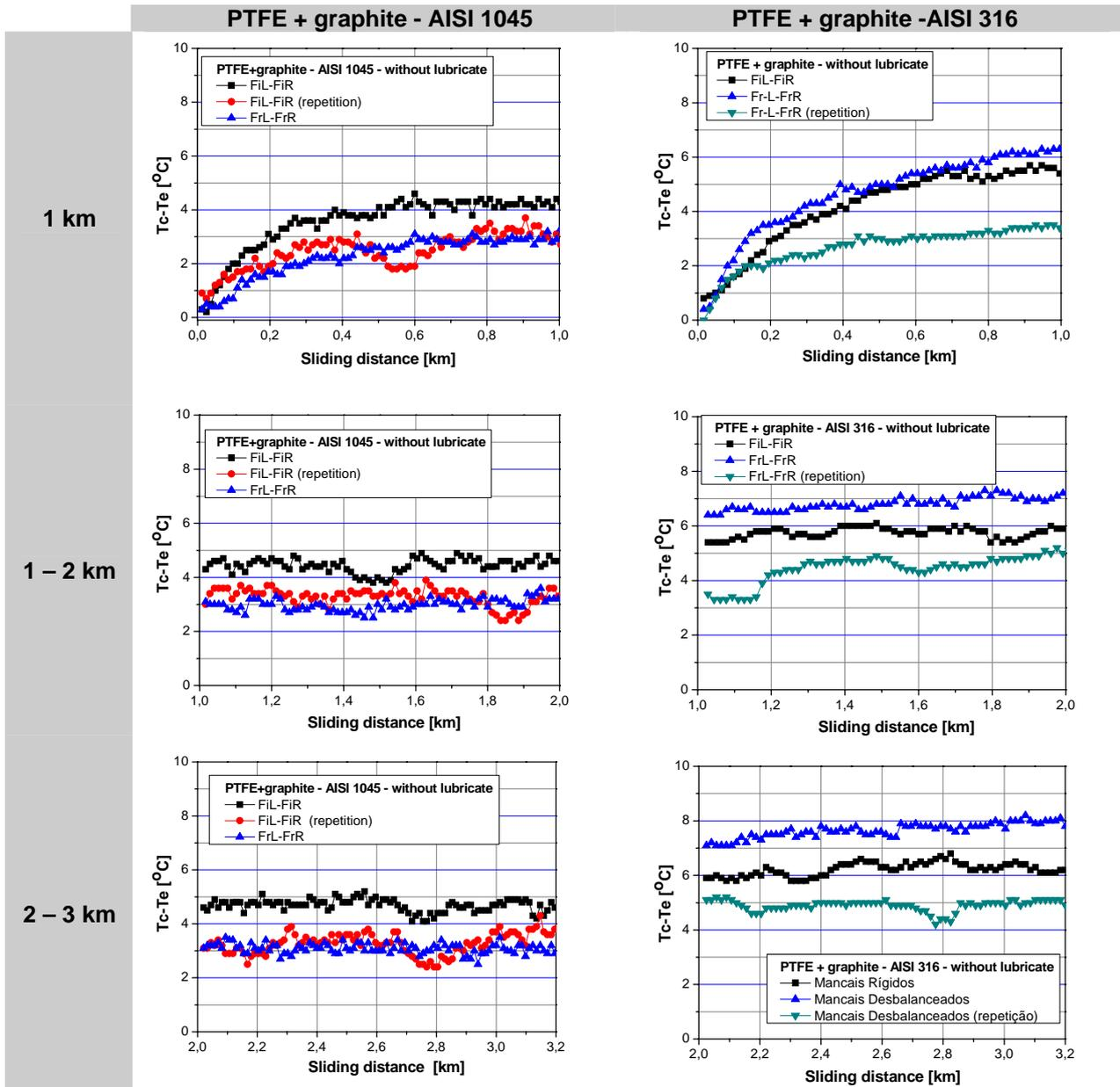
Figure 5. Variation of temperature next to the contact in the sliding testing to PTFE+graphite coupons against AISI 1045 and 316
