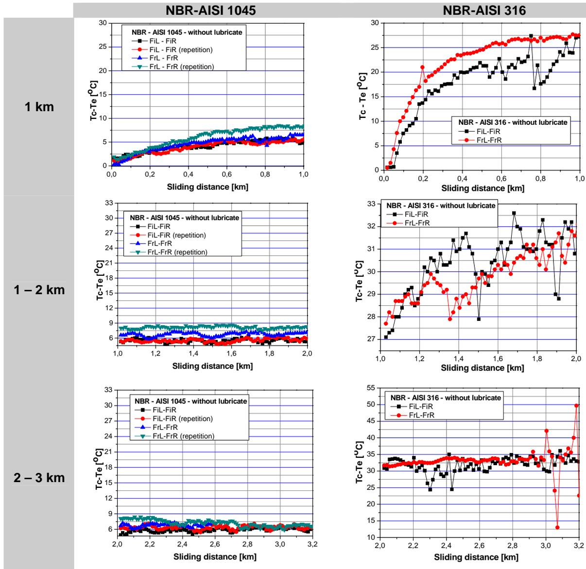
Figure 4. Variation of temperature next to the contact in the sliding testing to NBR coupons against AISI 1045 and 316
