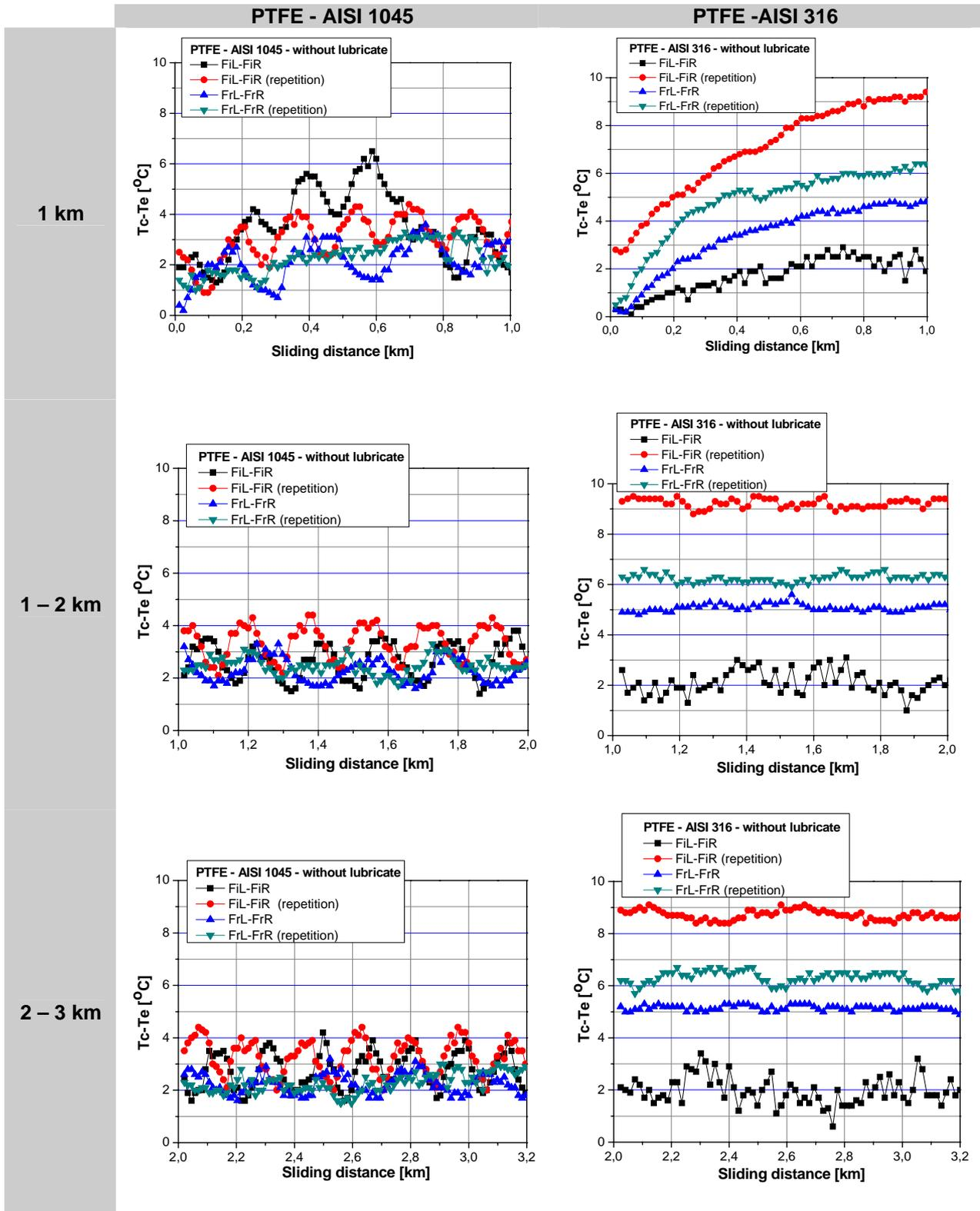
Figure 6. Variation of temperature next to the contact in the sliding testing to PTFE coupons against AISI 1045 and 316
