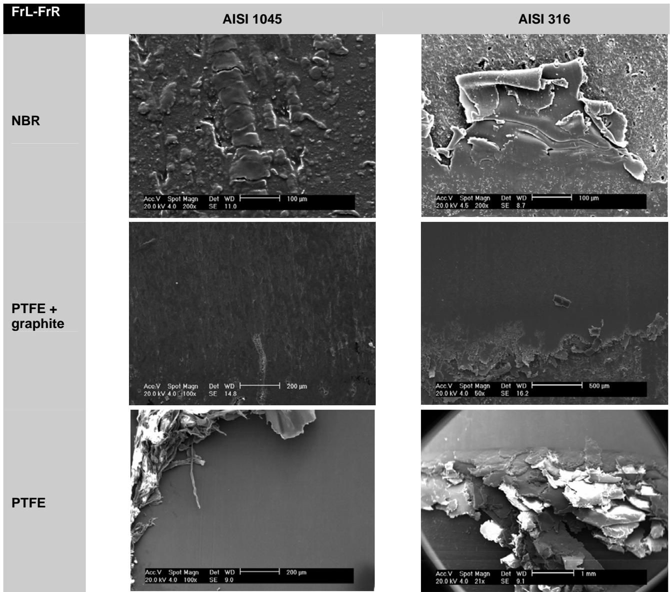
Figure 3. SEM micrographs from worn surface of the coupons after sliding against AISI 1045 and 316 steel in the FrL-FrR bearing configuration
