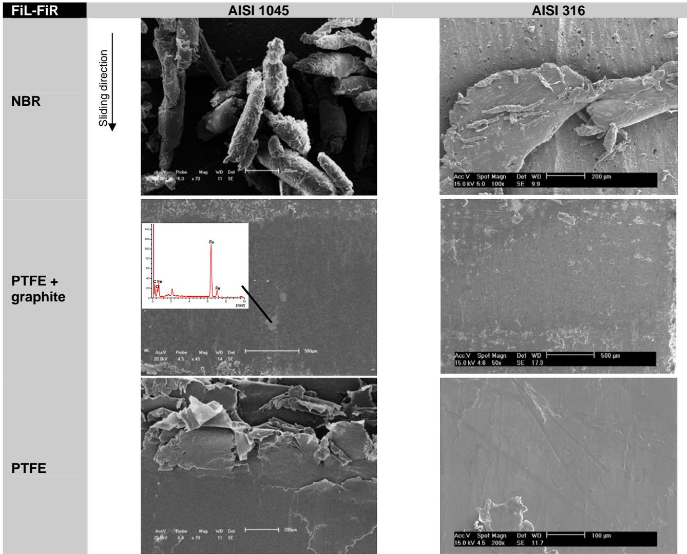
Figure 2. SEM micrographs from worn surface of the coupons after sliding against AISI 1045 and 316 steel in the FiL-FiR bearing configuration
