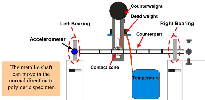
Figure 1. Schematic diagram of the sliding wear tester
