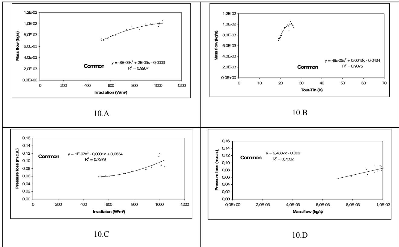
Figure 10. Dynamic behavior of solar collector of 30° tilt and 0.70 m of unevenness.
