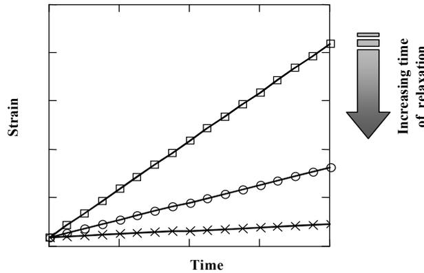
Figure 2. Maxwell model - creep response for different relaxation times
