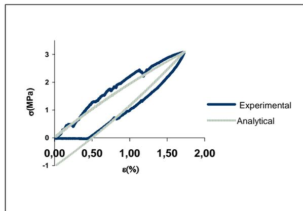
Figure 7. Stress x Strain - Analytical solution after identification process
