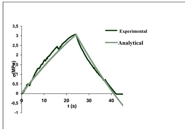
Figure 8. Stress x time - Analytical solution after identification process
