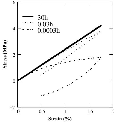
Figure 6. Initial viscosity estimated by Maxwell model from the creep test.
