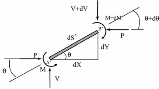
Figure 2. Infinitesimal element of the buckled rod.
