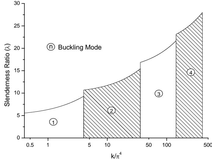
Figure 3. Slenderness Ratio as a function of the Foundation Stiffness.
