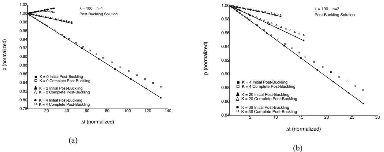
Figure 5. Normalized Load as a Function of the Normalized Temperature Gradient.
