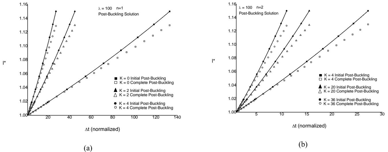
Figure 4. Strained Length as a Function of the Normalized Temperature Gradient.
