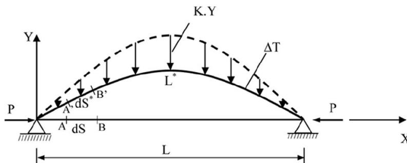
Figure 1. Rod initial and buckled forms on an elastic foundation.
