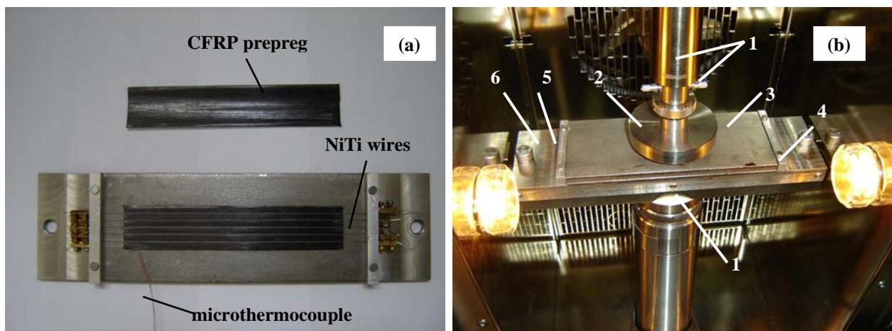
Figure 2. Pressure mold for manufacturing of sandwich CFRP-NiTi composite specimens. (a) Preparation for hot pressure molding. (b) Installation of the mold into the thermal chamber of the testing machine.
