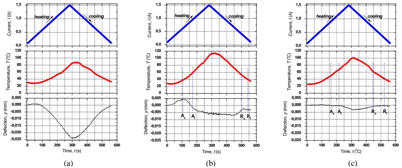
Figure 8. Thermal buckling of the CFRP-NiTi composites. (a) Cold-worked NiTi wires. (b) Annealed NiTi wires. (c) Trained NiTi wires.
