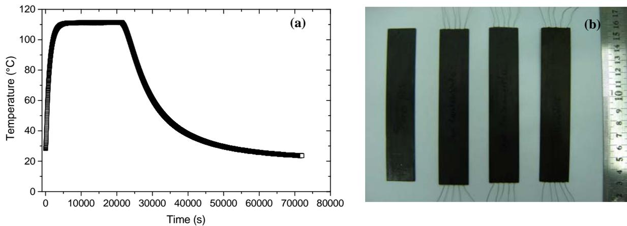
Figure 3. Fabrication of the CFRP-NiTi composites. (a) Temperature curing cycle. (b) Active composite beam specimens.
