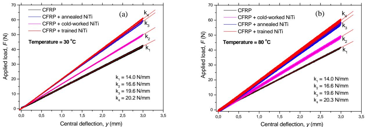
Figure 6. Thermomechanical behavior of the CFRP-NiTi active composites tested in a three point bending mode. Superposition of ten  $F - y$  cycles. (a) Test at 30  $^{\circ}\text{C}$ . (b) Test at 80  $^{\circ}\text{C}$ .
