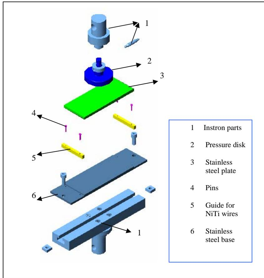
Figure 1. Design of the pressure molding system adapted in the 5582 Instron machine.
