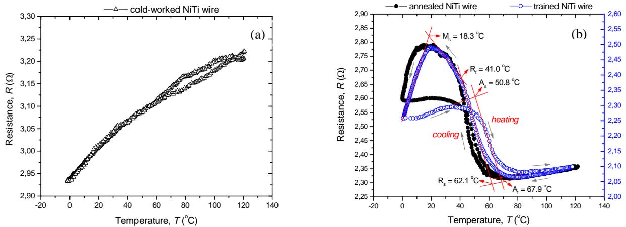
Figure 5. Phase transformation of the NiTi wires. (a) Cold-worked. (b) Annealed and trained.
