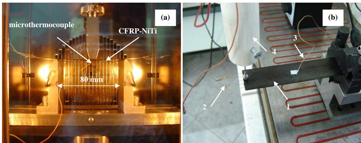
Figure 4. Assembly for testing the CFRP-NiTi active composites. (a) Three point bending tests. (b) Thermal buckling in cantilevered beam mode.
