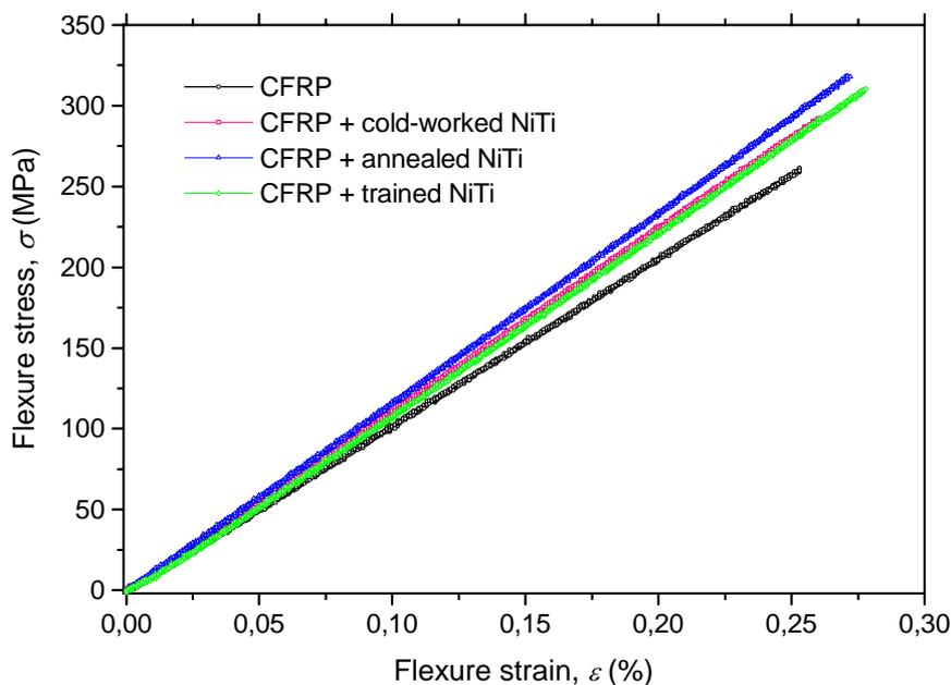
Figure 7. Mechanical behavior of the CFRP-NiTi specimens during three point bending tests at 30 °C.
