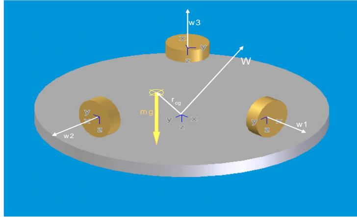
Figure 1 Satellite Attitude Control System Simulator Platform
