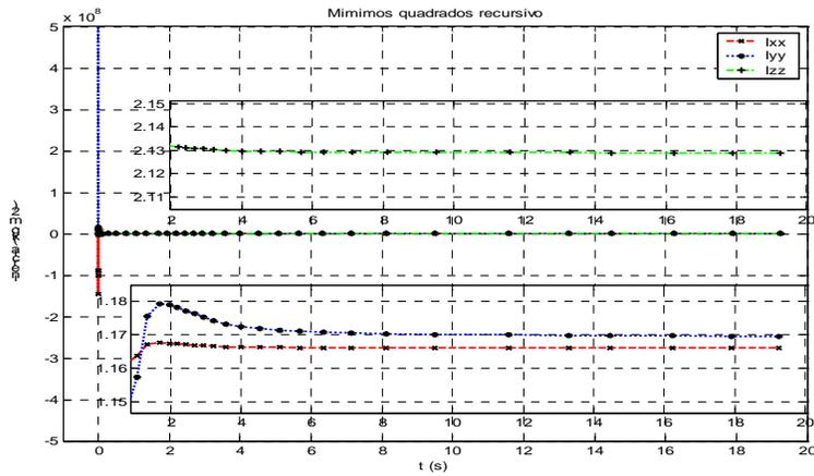
Figure 2 – Platform principal inertia parameters estimation
