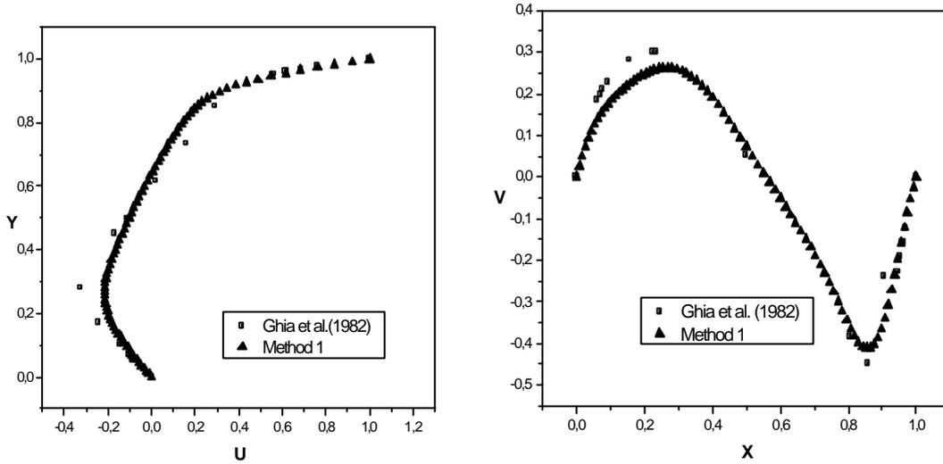
Figure 2: Method 1, Re= 400 (a) U-velocity at X = 0,5 (b) V-velocity at Y = 0,5
