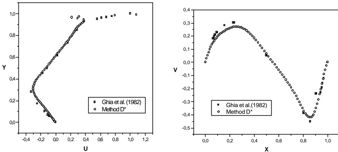
Figure 3: Method D\*, Re= 400 (a) U-velocity at X = 0,5 (b) V-velocity at Y = 0,5
