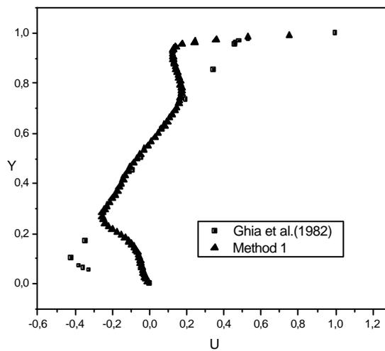
Figure 6: Method 1, Re= 3200, U-velocity at X = 0,5
