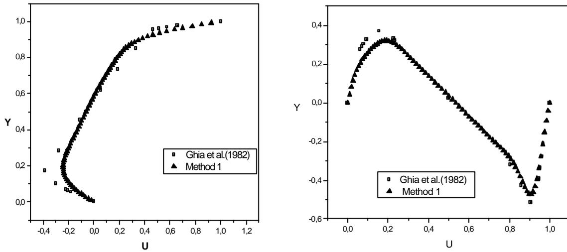
Figure 4: Method 1, Re= 1000 (a) U-velocity at X = 0,5 (b) V-velocity at Y = 0,5
