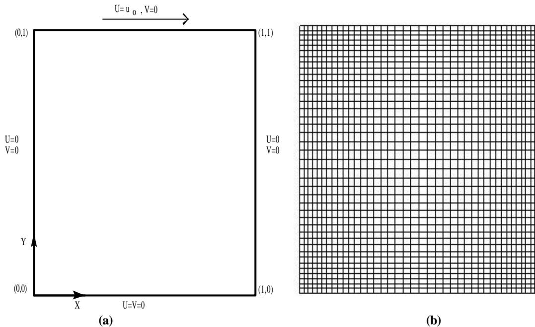
Figure 1 - Cavity flow: (a) configuration, coordinates and boundary conditions
