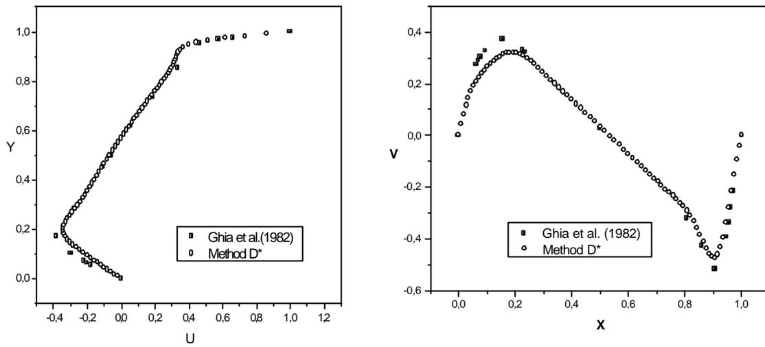
Figure 5: Method D\*, Re= 1000 (a) U-velocity at X = 0,5 (b) V-velocity at Y = 0,5
