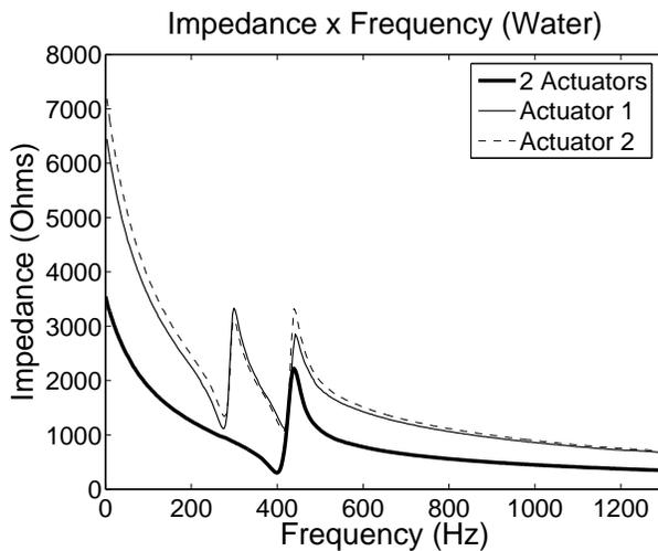
Figure 12. Impedance versus frequency curve in water.
