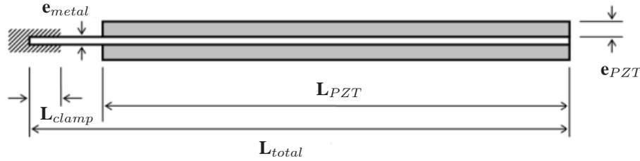
Figure 5. Geometric characteristics of the piezoactuator.
