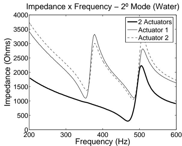
Figure 13. Impedance versus frequency curve in water. Detail for second mode.
