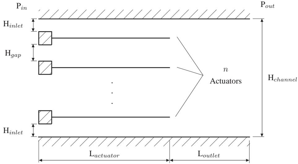
Figure 4. Piezoelectric flow pump with actuators in parallel configuration.
