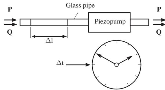
Figure 9. Apparatus for experimental flow rate characterization.
