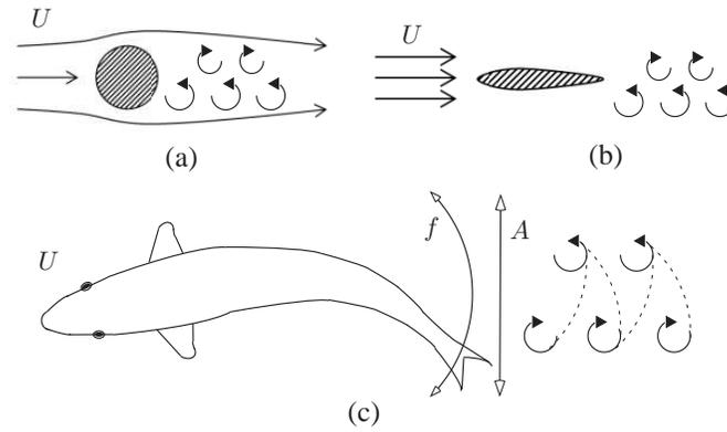
Figure 2. Karman street for a cylinder (a) and for a wing profile (b). Wake left by a fish swimming (c). The formation of an array of trailing discrete vortices of alternating signal is observed.
