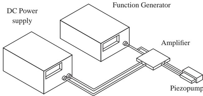
Figure 8. Piezoelectric pump driver apparatus.
