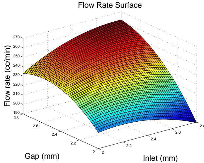
Figure 7. Flow rate surface obtained using the Response Surface Method.
