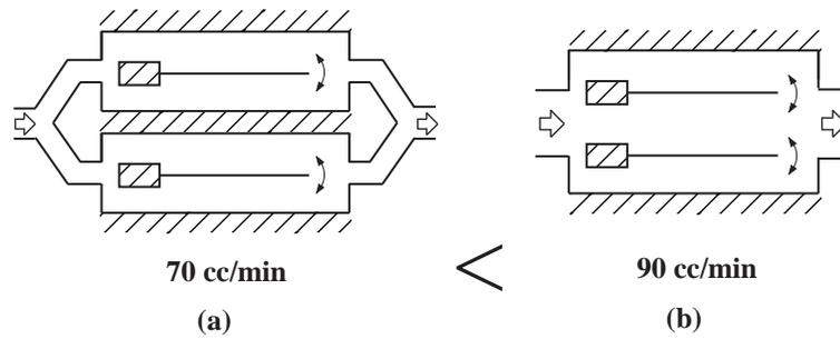
Figure 6. Two actuators in parallel configuration inside the same pump generate higher flow rate. (a) Two flow pumps with only one actuator in each one, (b) Flow pump with two actuators in parallel configuration.
