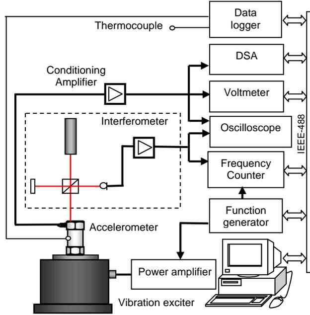
Figure 1: Interferometric calibration system - Fringe counting method
