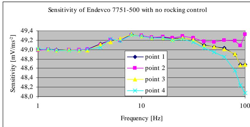
Fig. 9: Sensitivity of the Endevco 7751-500 calculated at each measurement point.
