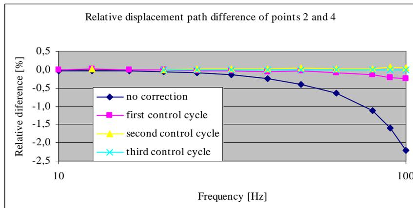
Fig. 11: Relative displacement between points 2 and 4.
