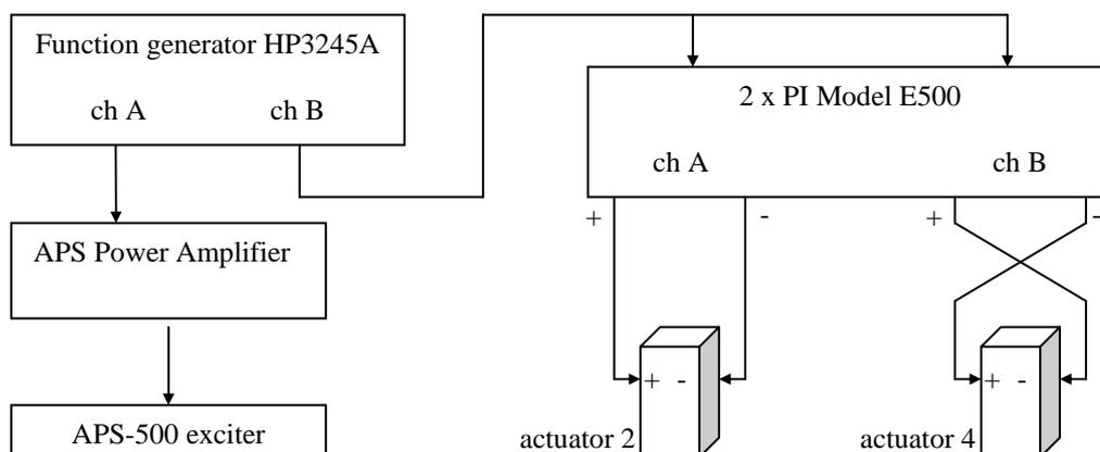
Fig 6: Electrical connections of the piezoelectric actuators.
