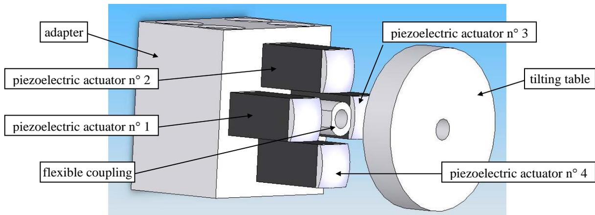
Fig. 2: Actuation system. The tilting table is moved to show the actuators.
