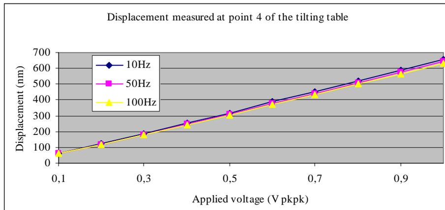
Fig. 8: Calibration of tilting table rotation versus applied voltage.
