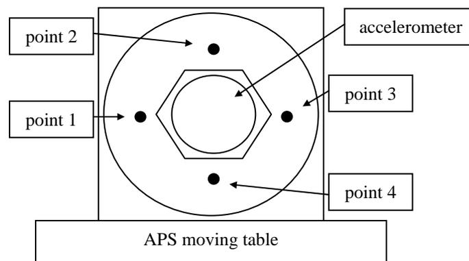
Fig. 7: Location of the measurement points.
