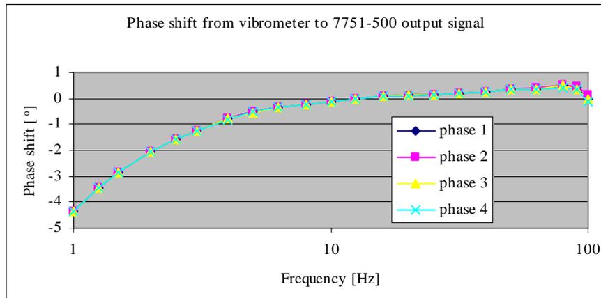
Fig. 10: Phase shift of the Endevco 7751-500 and vibrometer signals at each measurement point.
