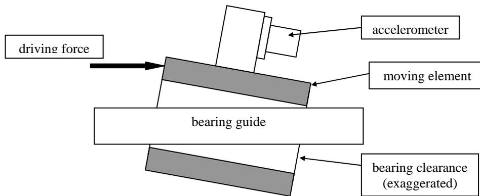
Fig. 5: Effect of the bearing clearance over the accelerometer.
