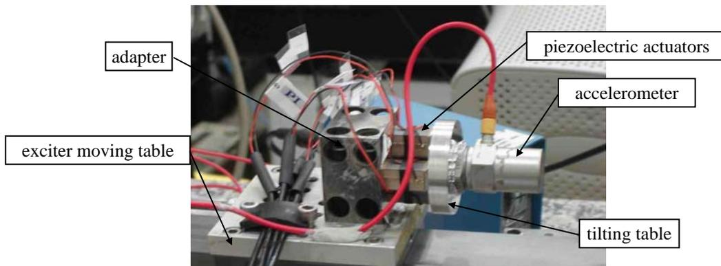
Fig. 3: View of the system mounted over the APS exciter.
