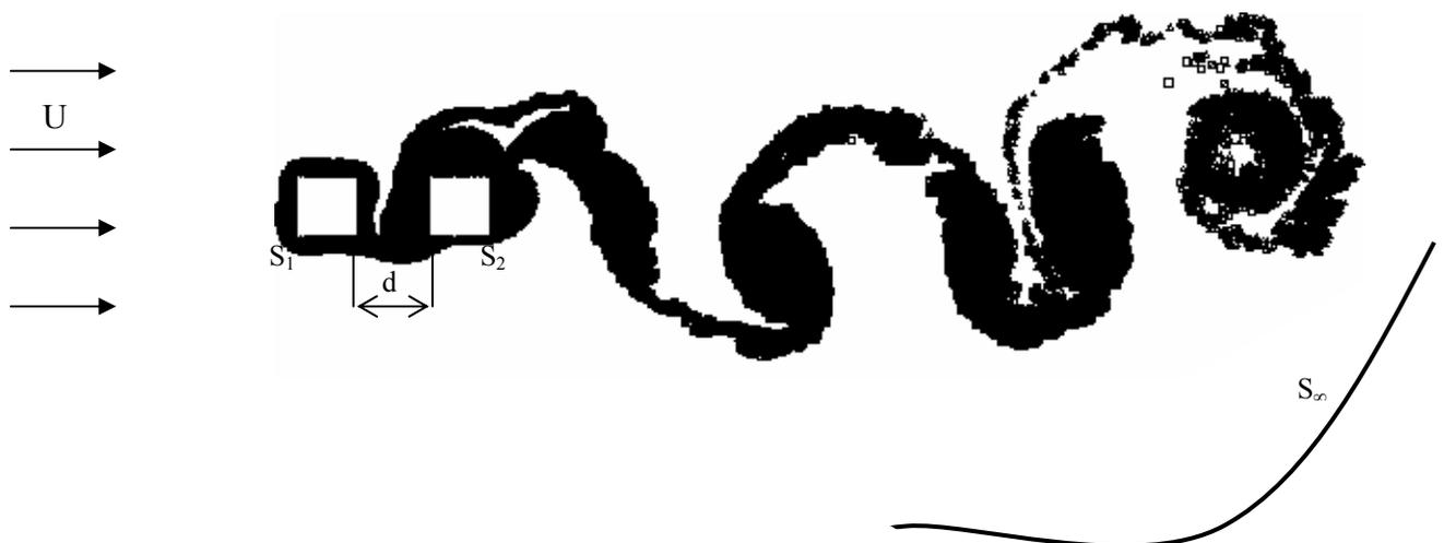
Figure 1. Flow around two square cylinders in a tandem arrangement.
