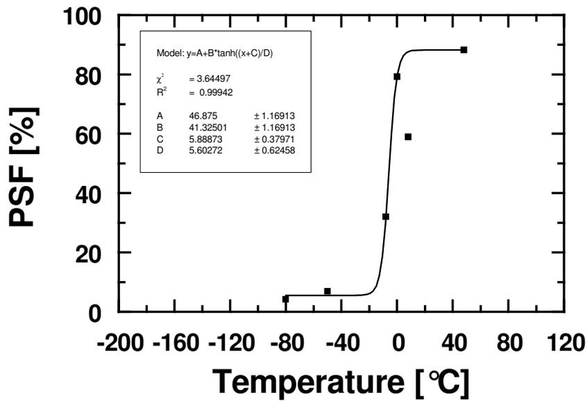
Figure 10 – Percentage of shear fracture (PSF) obtained from analysis surface fracture to T-L direction for ABNT 1016 steel.
