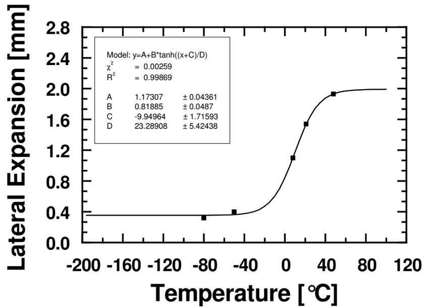
Figure 7 – Curve lateral expansion-temperature of L-T direction for 1016 ABNT steel.
