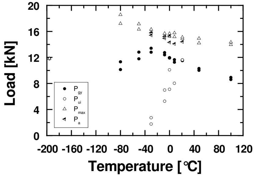
Figure 12 – Load diagram in L-T direction for ABNT 1016 steel.
