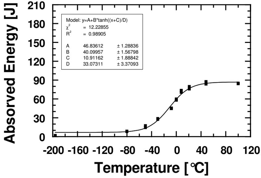
Figure 5 – Curve energy-temperature of L-T direction for 1016 ABNT steel.
