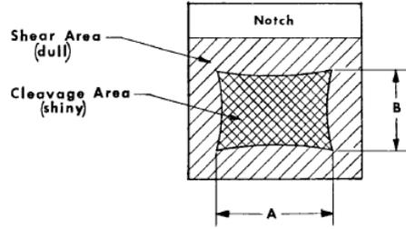
Figure 3 – Fracture surface of a Charpy V-notch impact specimen. (ASTM-E23, 2005)
