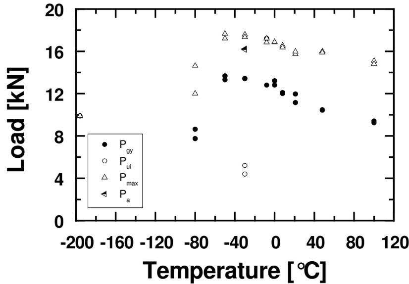
Figure 13 – Load diagram in T-L direction for ABNT 1016 steel.
