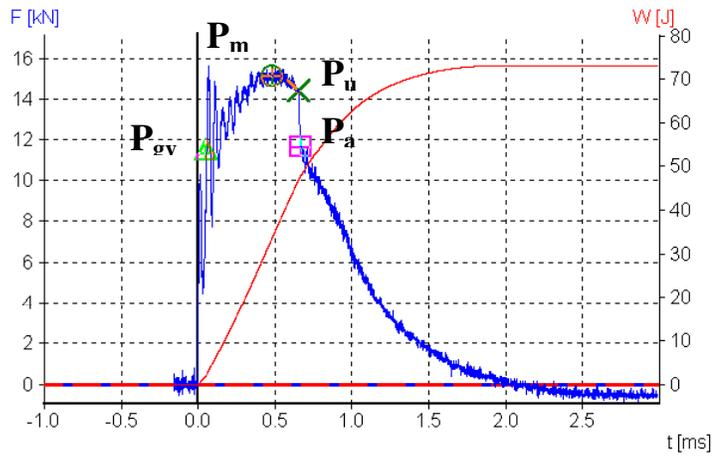
Figure 11 - Curves load-time and energy-time were obtained by instrumented impact Charpy test in transition region for ABTN 1016 steel.  $P_{gy}$  was corresponded transition elastic-plastic,  $P_m$  was maximum load,  $P_u$  was beginning unstable crack and  $P_a$  was beginning lateral expansion.
