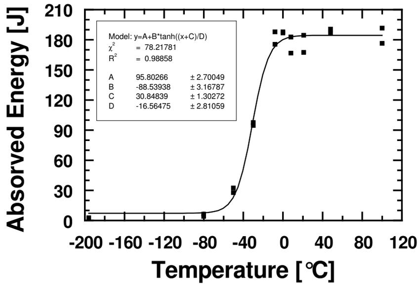
Figure 6 – Curve energy-temperature of T-L direction for 1016 ABNT steel.
