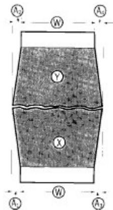
Figure 2 – Halves of broken Charpy V-notch impact specimen. (ASTM-E23, 2005)
