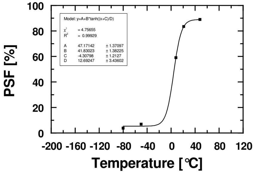
Figure 9 – Percentage of shear fracture (PSF) obtained from analysis surface fracture to L-T direction for ABNT 1016 steel.
