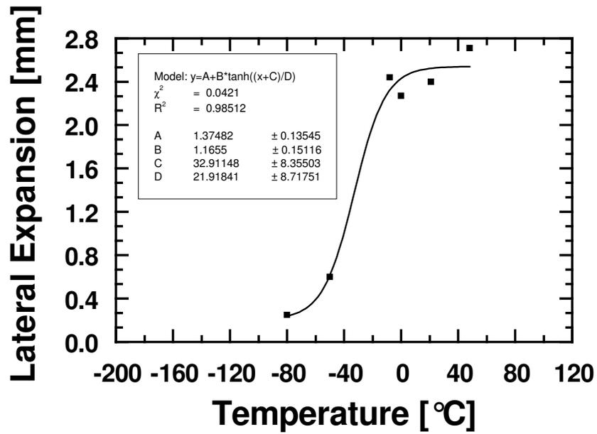
Figure 8 – Curve lateral expansion-temperature of T-L direction for 1016 ABNT steel.
