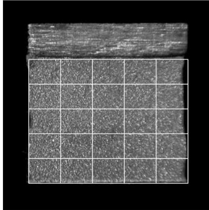
Figure 4 – Mesh on the fracture area. (Cochrane, 2007)
