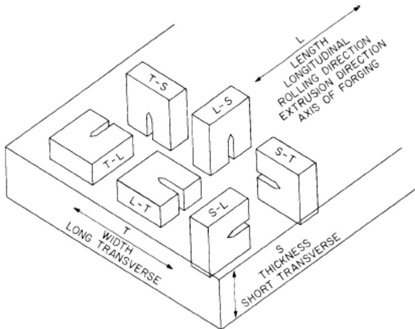
Figure 1 – Crack plane orientation code for rectangular sections. (ASTM-E399, 1997)
